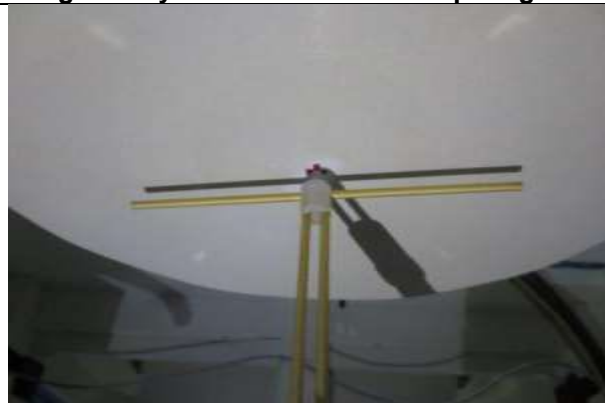
Fig.10.2 Photo of Dipole setup
