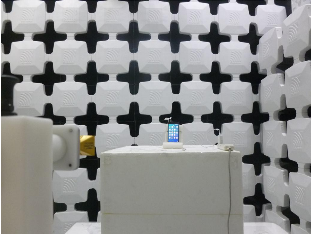
Radiated Spurious Emissions Test Setup Above 1GHz
