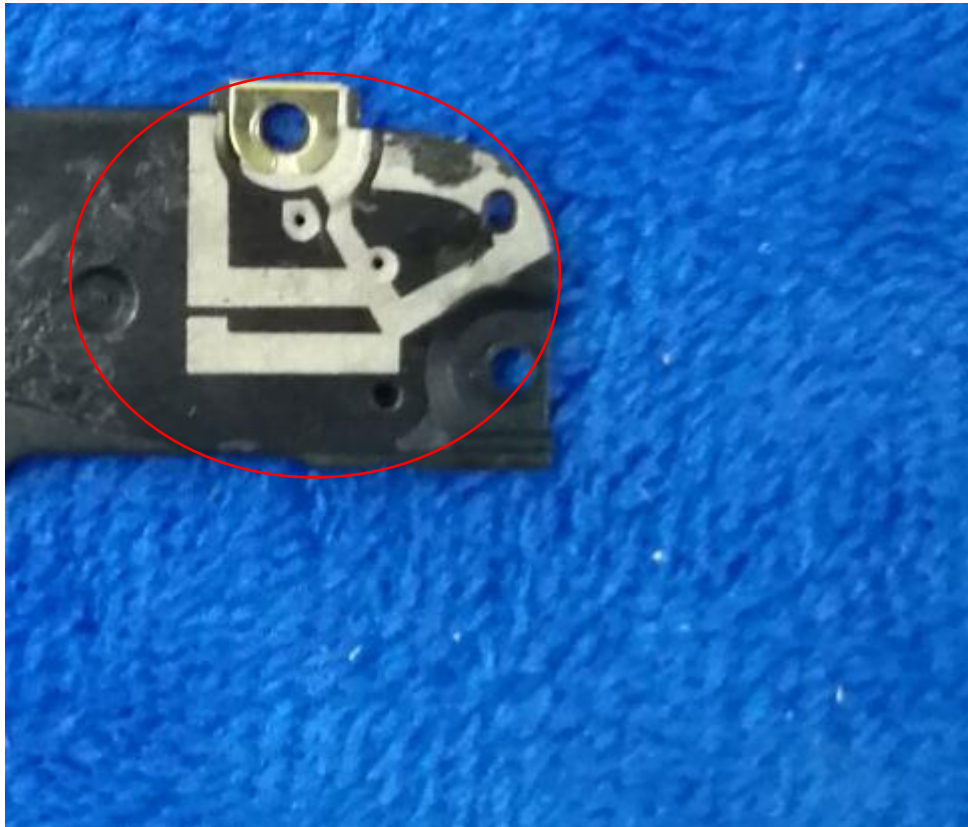
2.4WIFI/5G WIFI/BT/BLE/GPS - Antenna View
