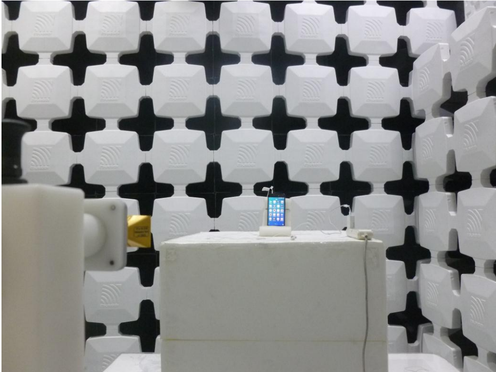
Radiated Spurious Emissions Test Setup Above 1GHz
