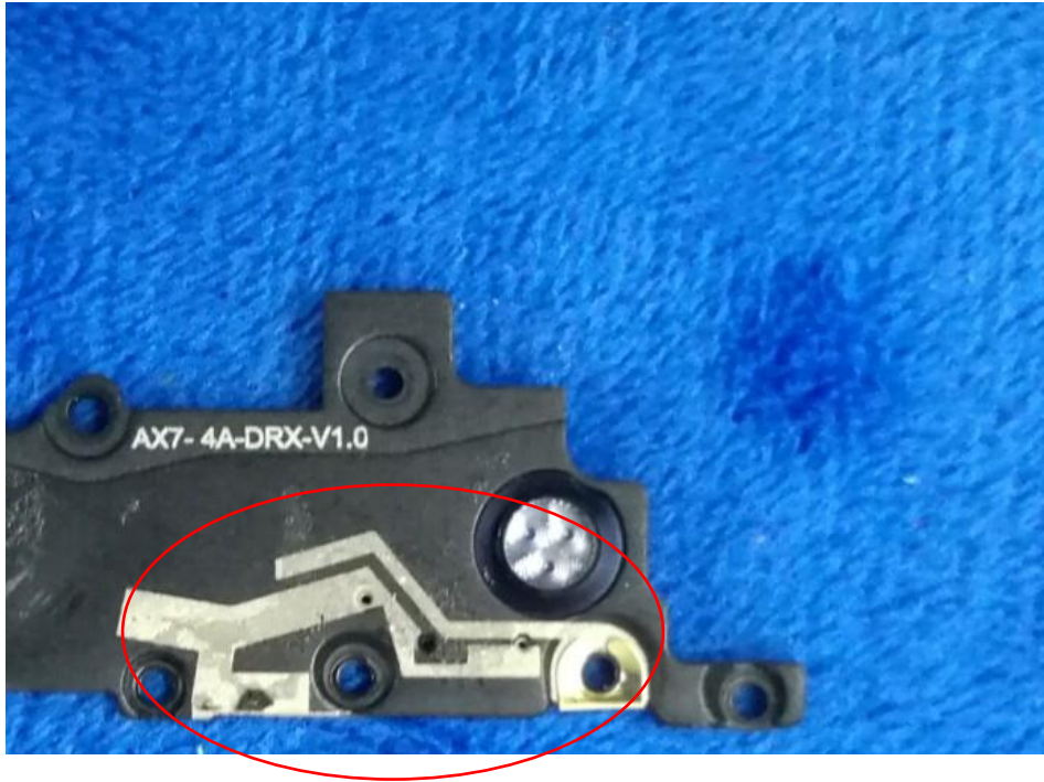
LTE - Antenna View
