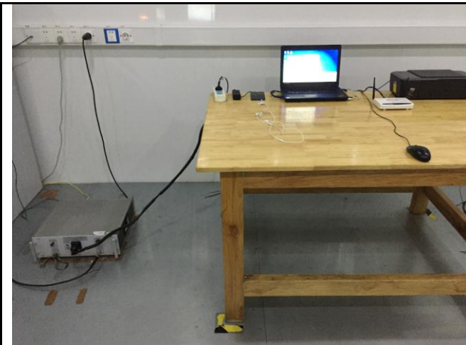
Conducted Emissions Test Setup – Front View
