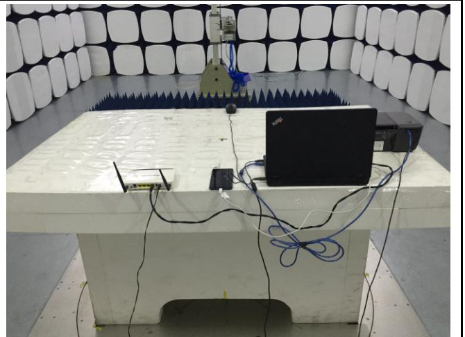
Radiated Emissions Test Setup Above 1GHz
