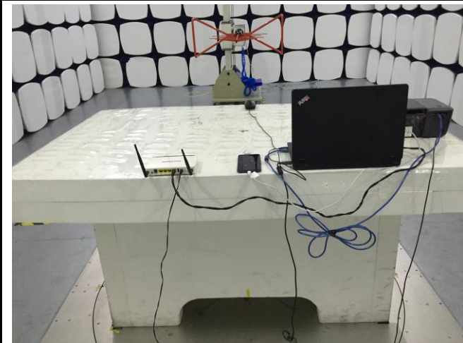
Radiated Emissions Test Setup Below 1GHz
