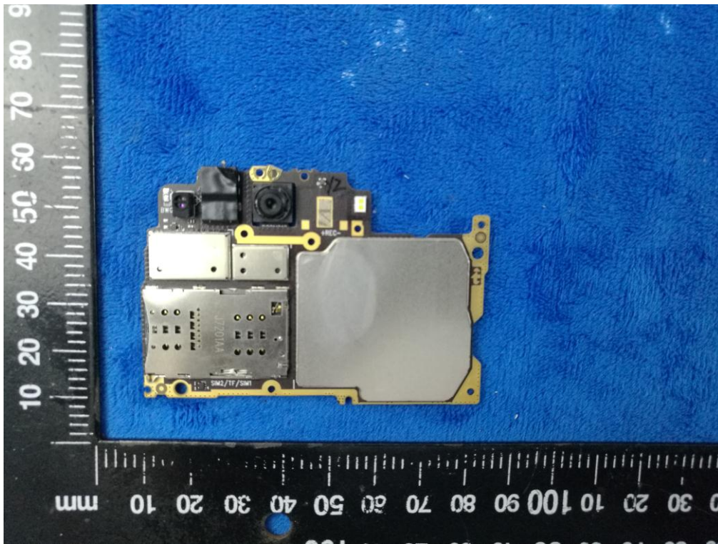
Mainboard with Shielding- Rear View
