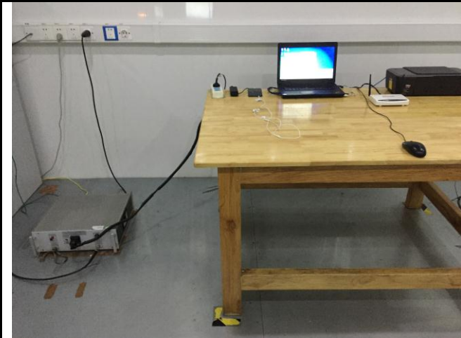
Conducted Emissions Test Setup – Front View
