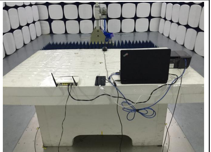
Radiated Emissions Test Setup Above 1GHz
