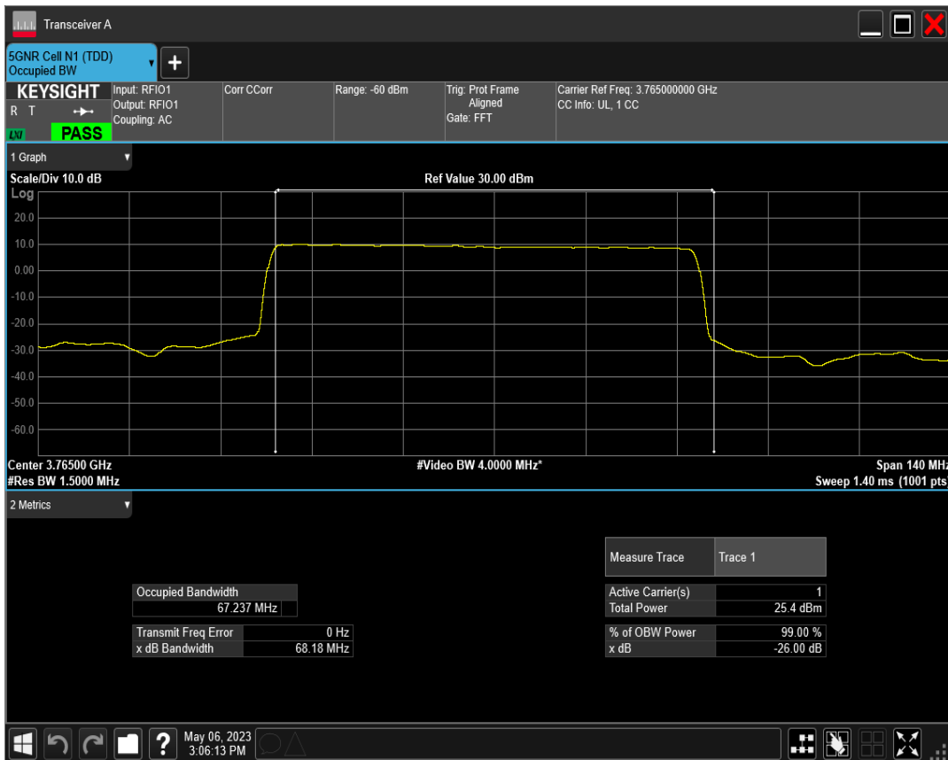
n78(3700-3800) SCS=30kHz DFT_QPSK BW=70MHz Channel=651000 RB=180@0
