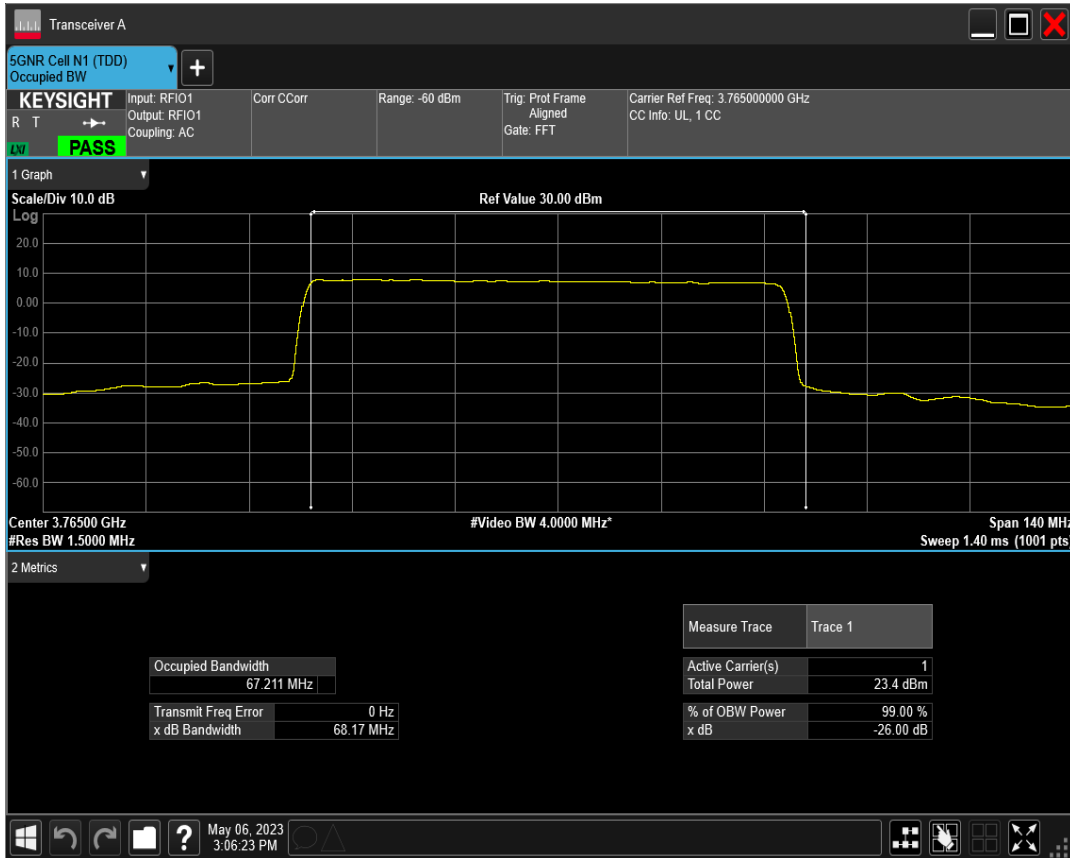
n78(3700-3800) SCS=30kHz CP_QPSK BW=70MHz Channel=651000 RB=189@0
