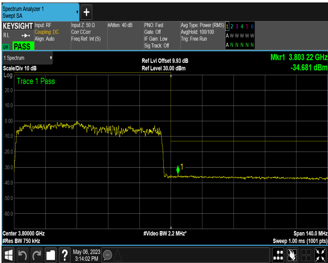
n78(3700-3800) SCS=30kHz DFT_QPSK BW=70MHz Channel=651000 RB=1@188
