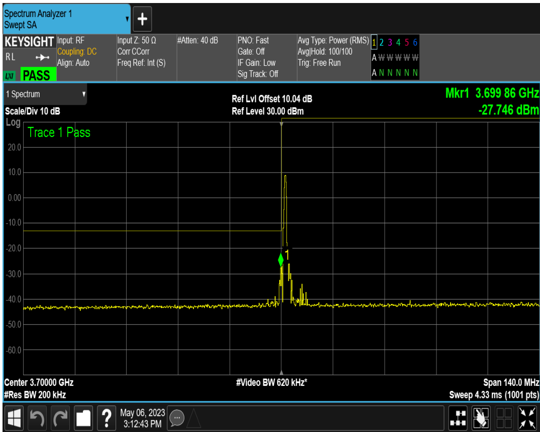
n78(3700-3800) SCS=30kHz DFT_QPSK BW=70MHz Channel=651000 RB=180@0
