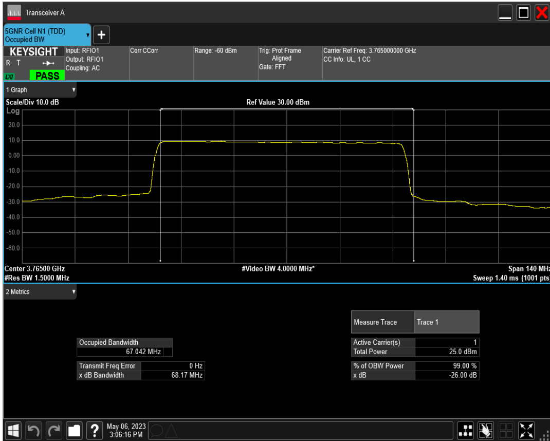
n78(3700-3800) SCS=30kHz DFT_QAM16 BW=70MHz Channel=651000 RB=180@0
