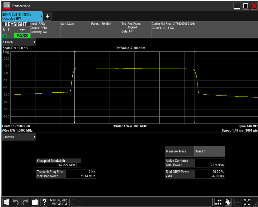
n78(3700-3800) SCS=30kHz DFT_BPSK BW=70MHz Channel=651000 RB=180@0
