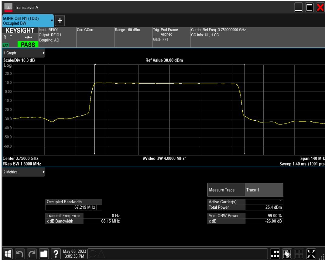
n78(3700-3800) SCS=30kHz DFT_QPSK BW=70MHz Channel=650000 RB=180@0
