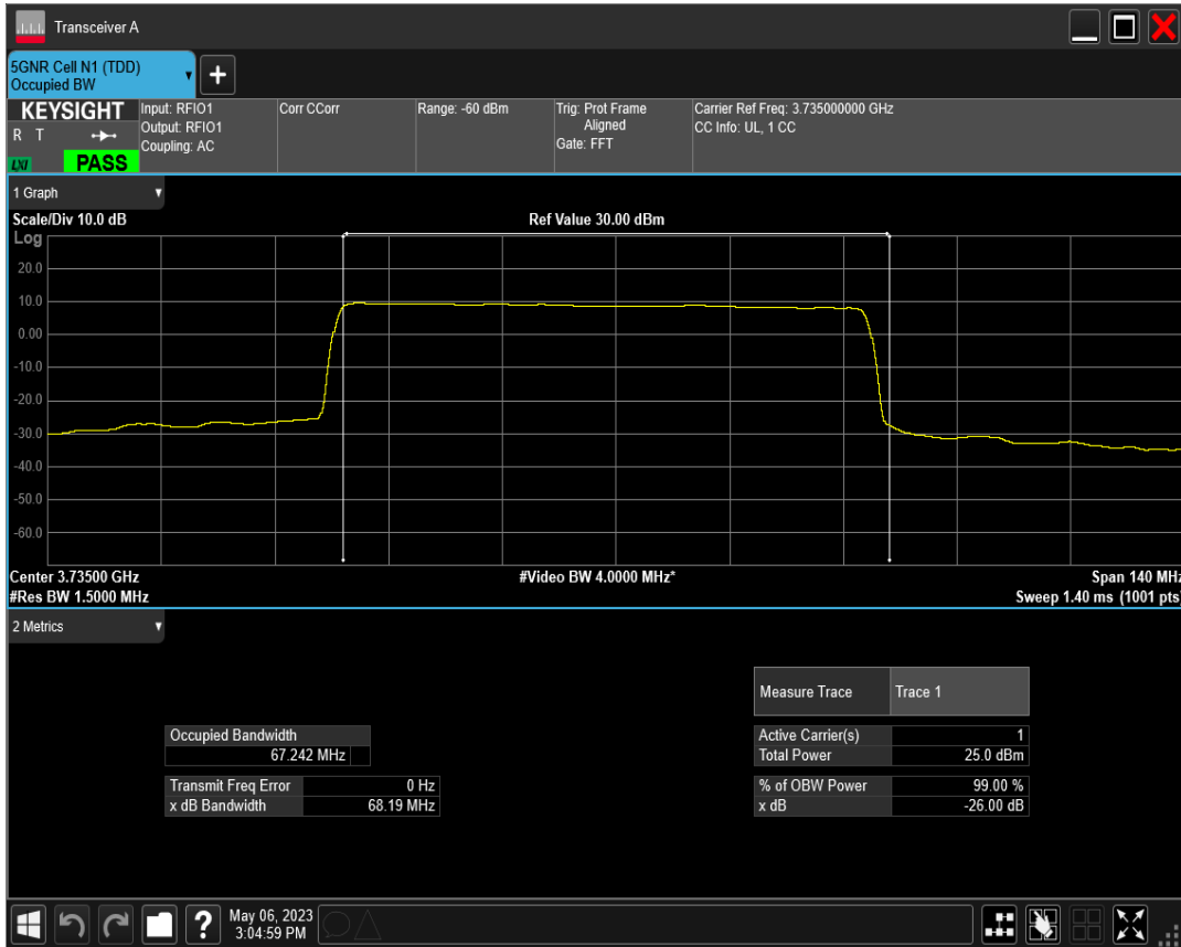
n78(3700-3800) SCS=30kHz DFT_QAM16 BW=70MHz Channel=649000 RB=180@0
