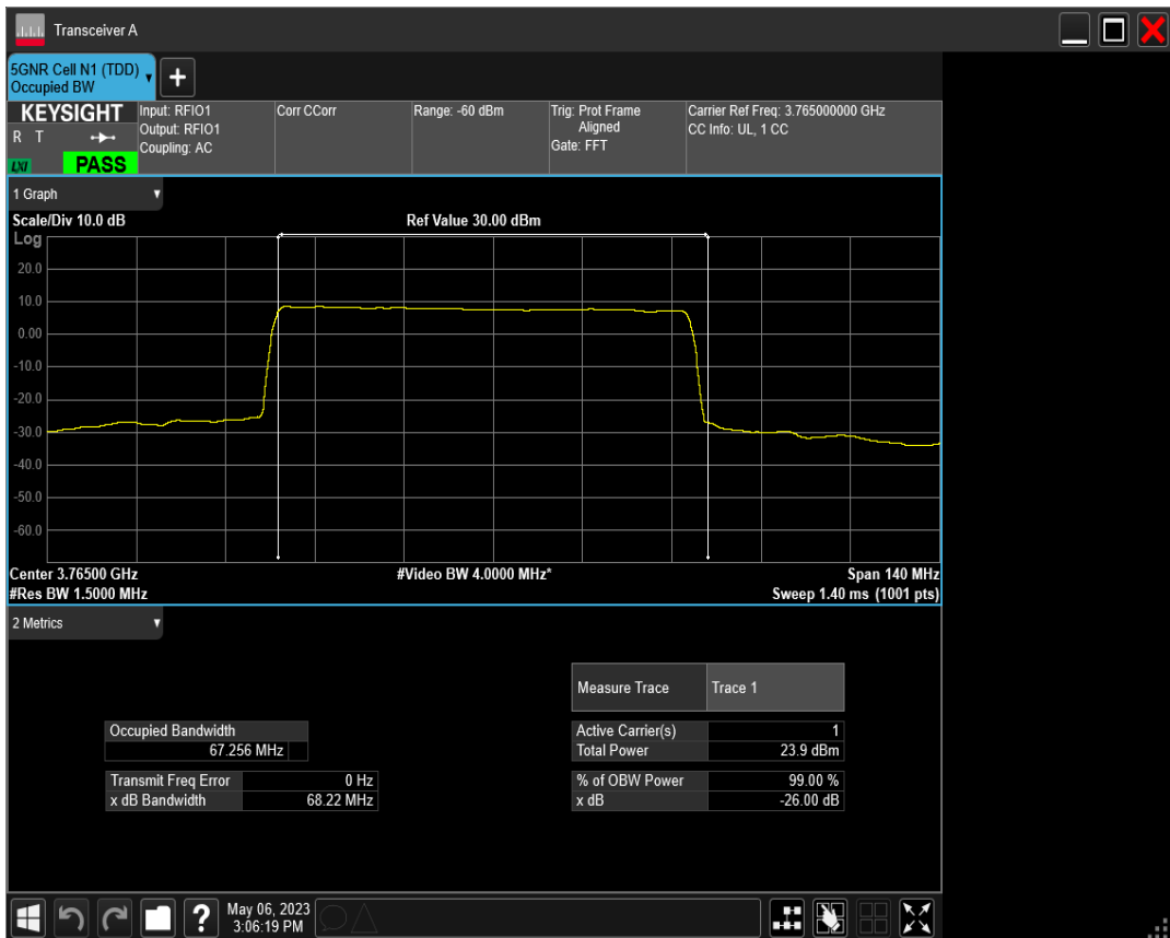
n78(3700-3800) SCS=30kHz DFT_QAM64 BW=70MHz Channel=651000 RB=180@0
