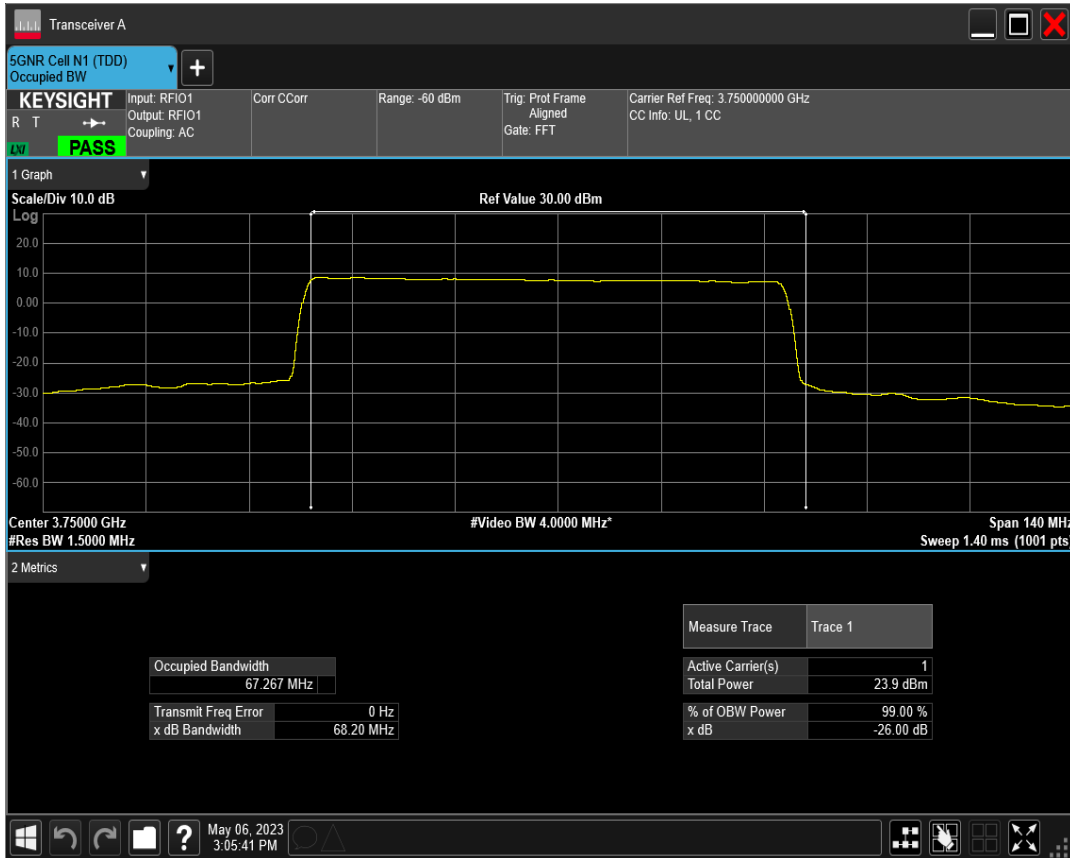
n78(3700-3800) SCS=30kHz DFT_QAM64 BW=70MHz Channel=650000 RB=180@0
