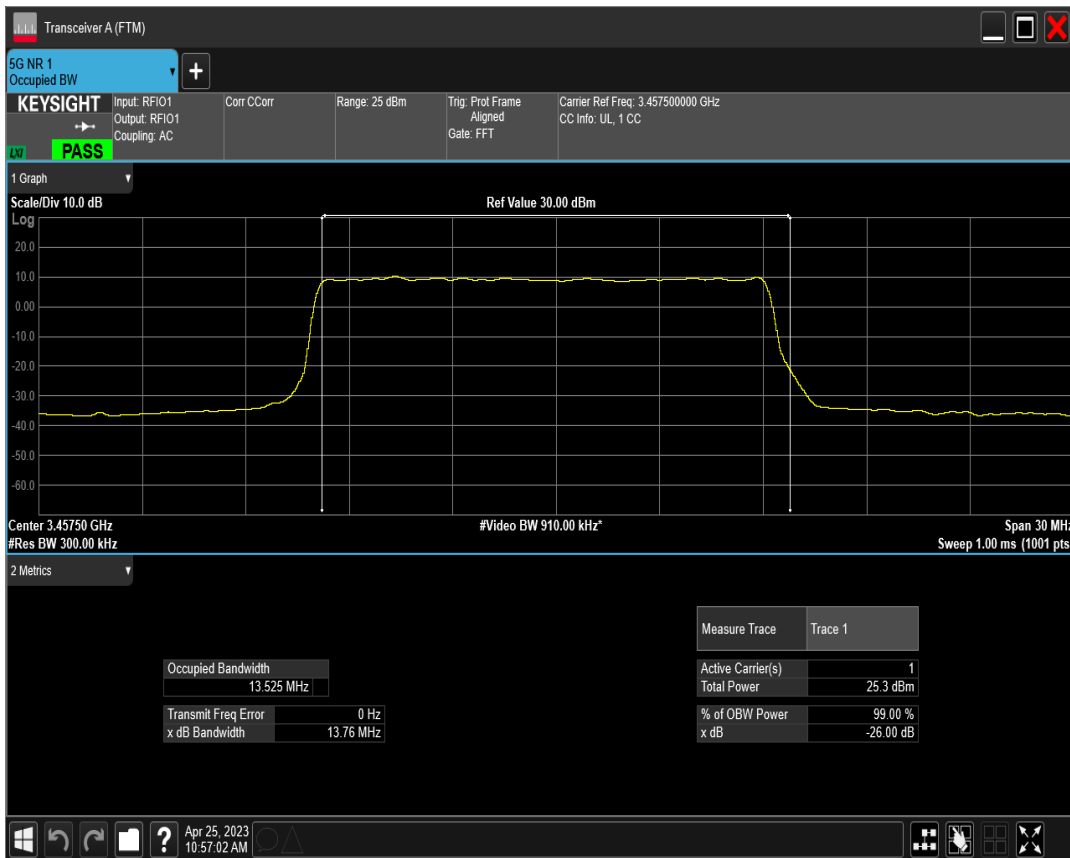
n77(3450-3550) SCS=30kHz DFT_QAM16 BW=15MHz Channel=630500 RB=36@0
