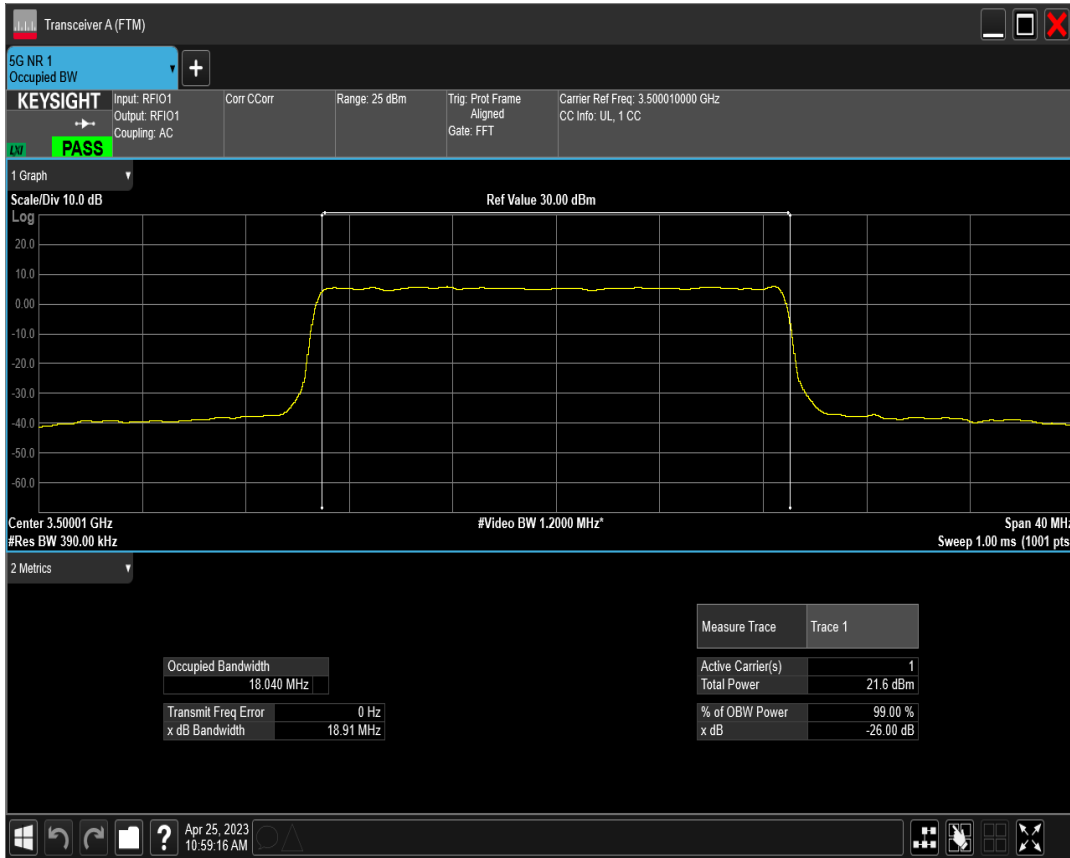
n77(3450-3550) SCS=30kHz CP_QPSK BW=20MHz Channel=633334 RB=51 @0
