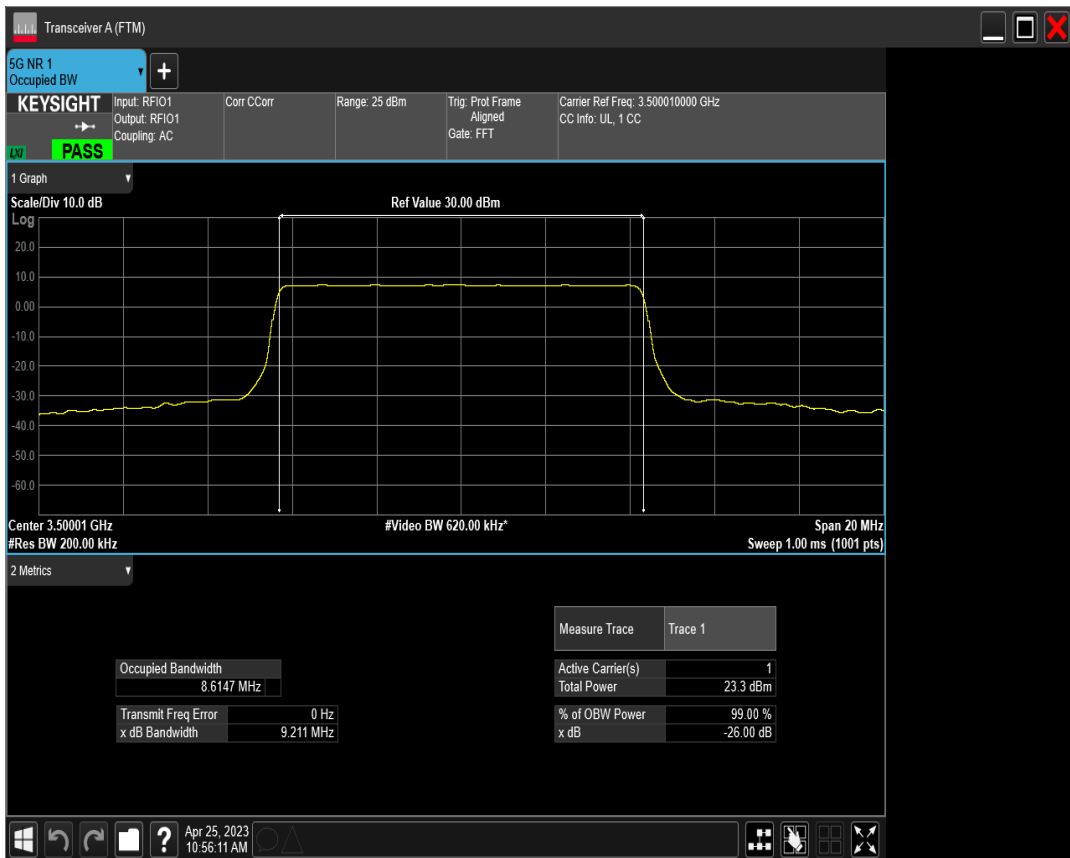
n77(3450-3550) SCS=30kHz DFT_BPSK BW=10MHz Channel=636332 RB=24@0
