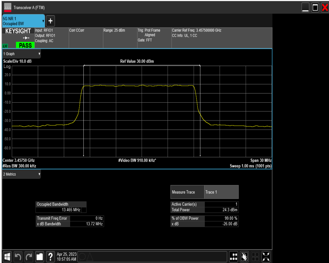
n77(3450-3550) SCS=30kHz DFT_QAM64 BW=15MHz Channel=630500 RB=36@0
