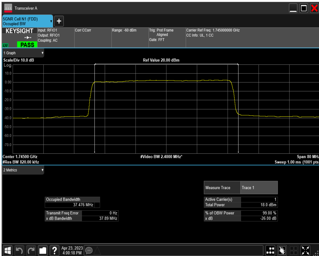
n66 SCS=30kHz DFT_QAM16 BW=40MHz Channel=349000 RB=100@0
