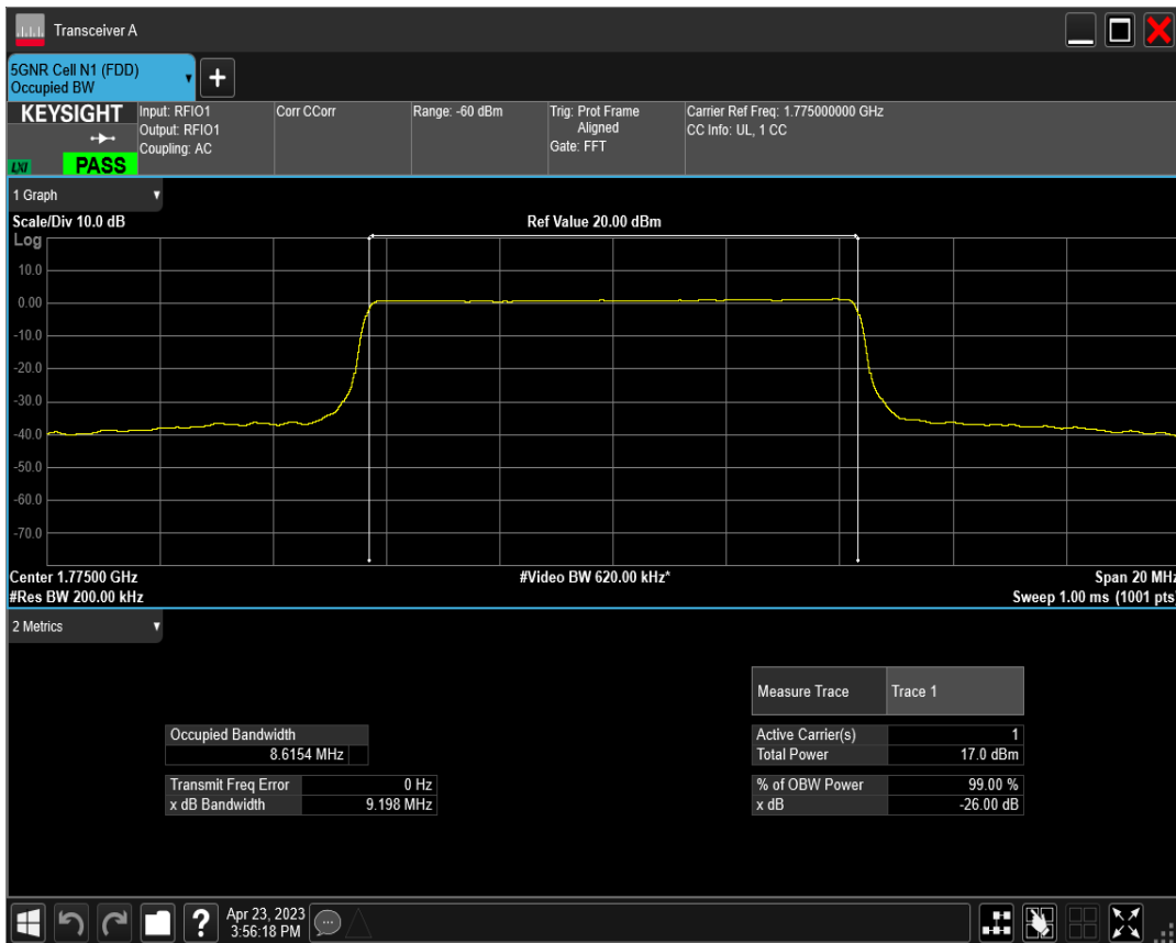
n66 SCS=30kHz DFT_BPSK BW=15MHz Channel=343500 RB=36@0
