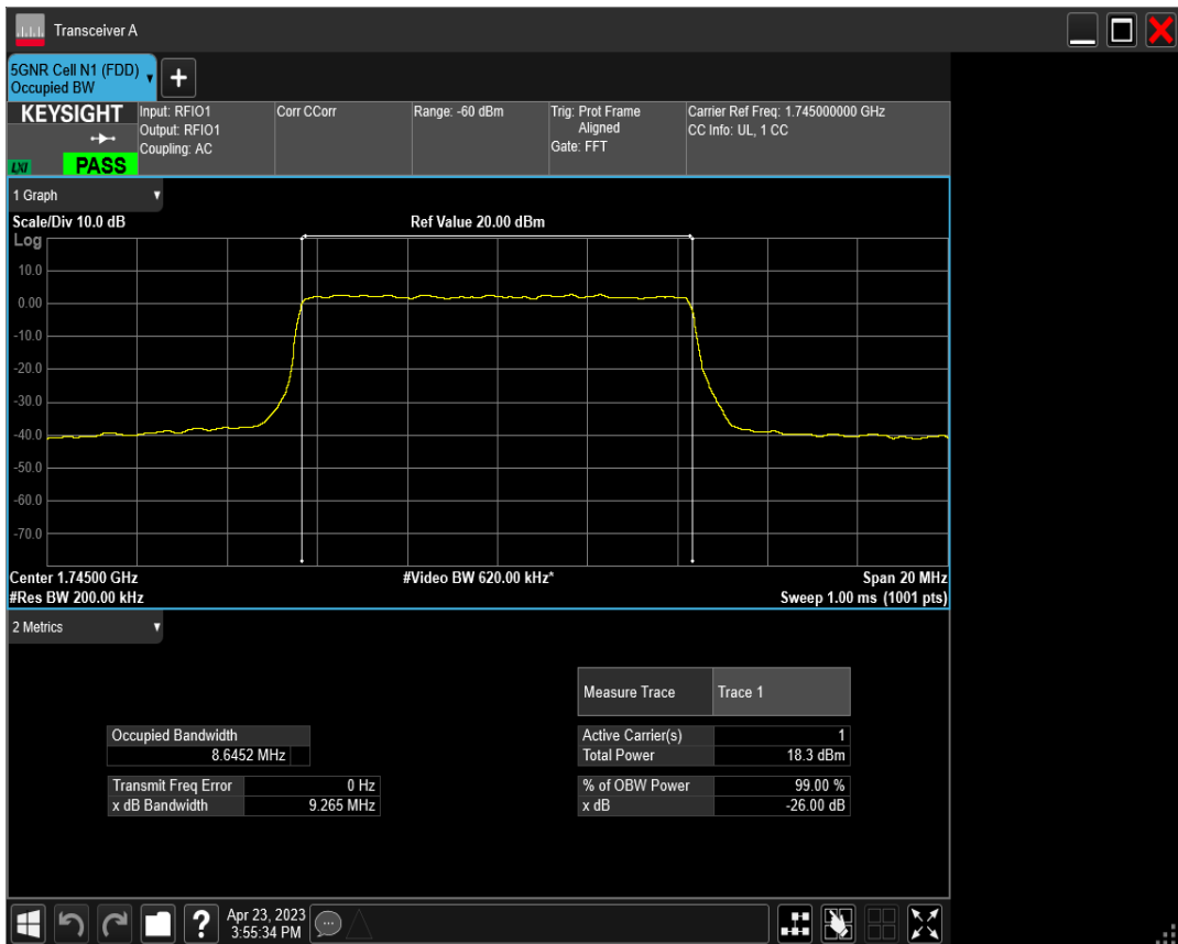
n66 SCS=30kHz DFT_QAM16 BW=10MHz Channel=349000 RB=24@0
