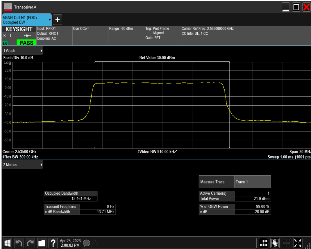
n7 SCS=30kHz DFT_QAM16 BW=15MHz Channel=507000 RB=36@0
