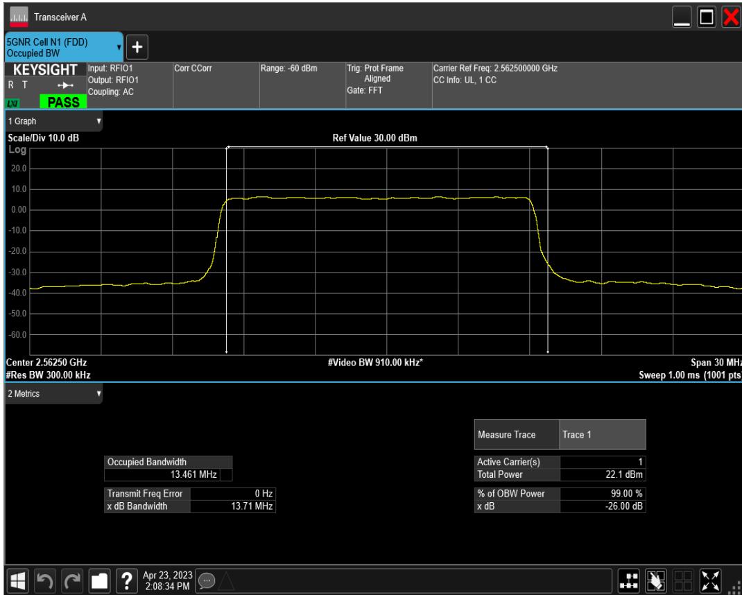
n7 SCS=30kHz DFT_QAM16 BW=15MHz Channel=512500 RB=36@0
