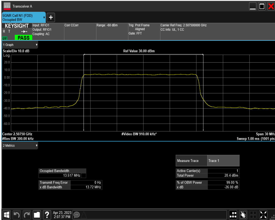
n7 SCS=30kHz DFT_QAM256 BW=15MHz Channel=501500 RB=36@0
