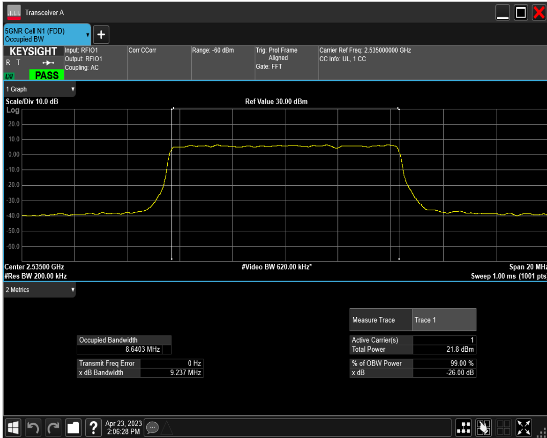
n7 SCS=30kHz DFT_QAM16 BW=10MHz Channel=507000 RB=24@0
