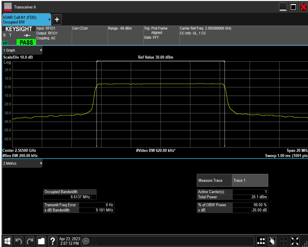
n7 SCS=30kHz DFT_BPSK BW=15MHz Channel=501500 RB=36@0
