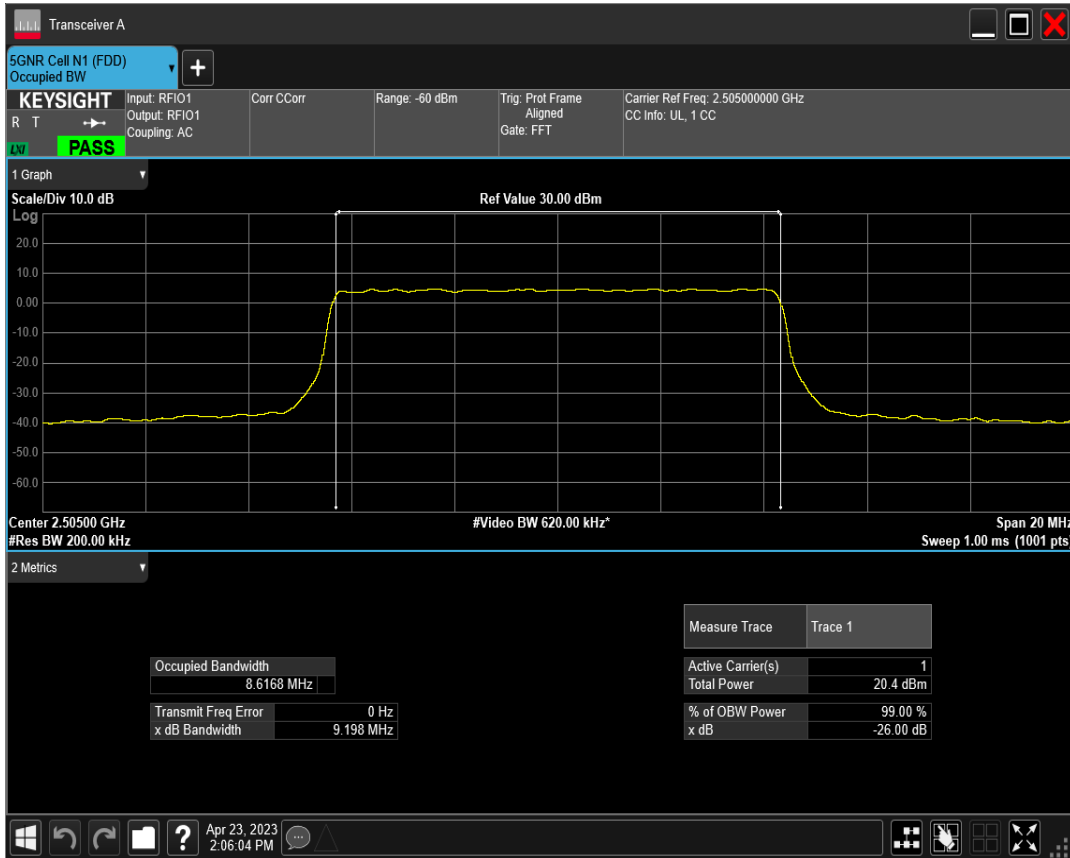
n7 SCS=30kHz DFT_QAM256 BW=10MHz Channel=501000 RB=24@0
