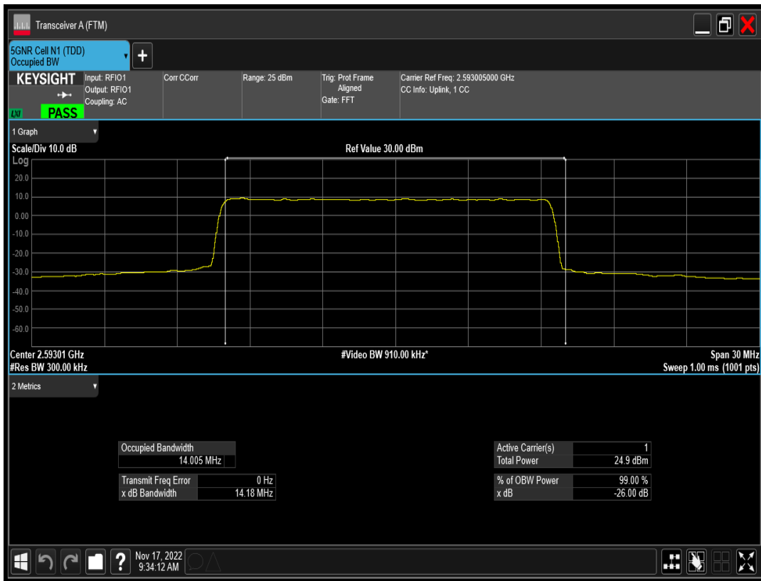
n41 SCS=15kHz DFT_QAM64 BW=15MHz Channel=518601 RB=75@0
