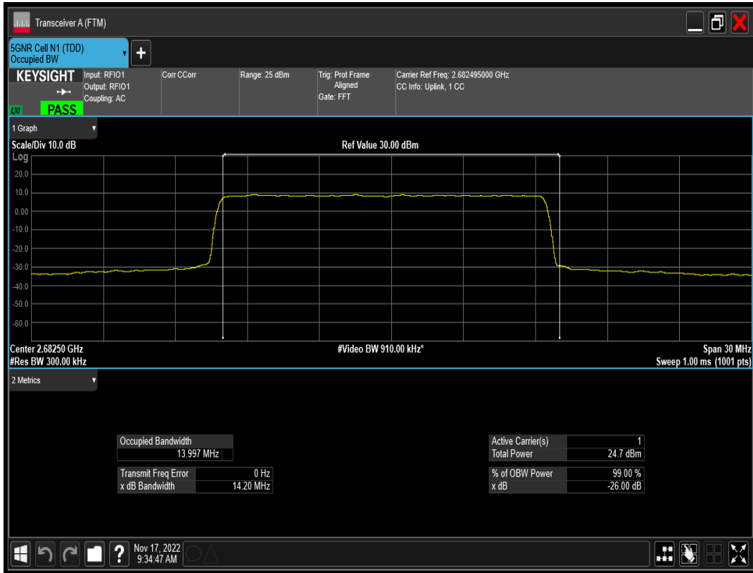
n41 SCS=15kHz DFT_QAM64 BW=15MHz Channel=536499 RB=75@0
