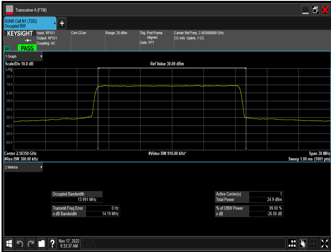
n41 SCS=15kHz DFT_QAM64 BW=15MHz Channel=500700 RB=75@0
