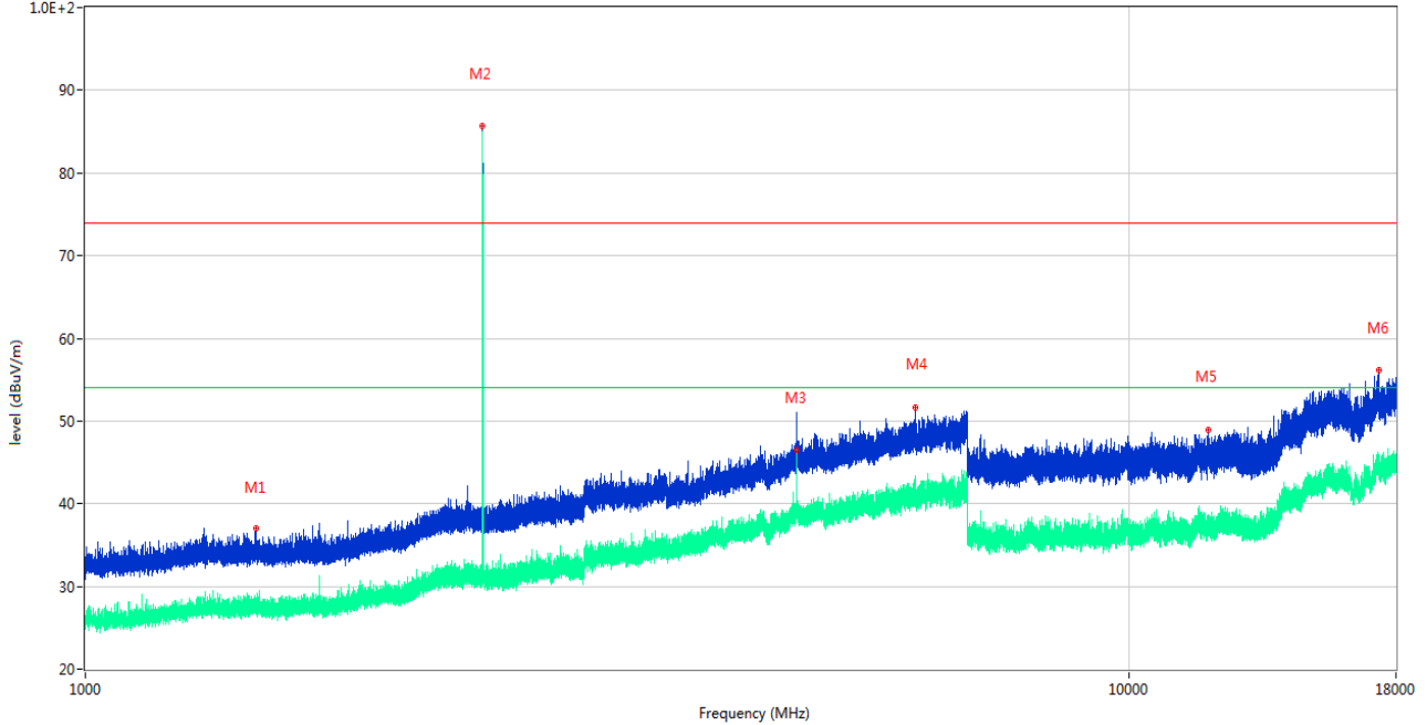
RE Test case_FCC Part 15C_FCC 15.247(2.4G)_1GHz-18GHz
