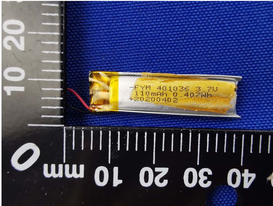
Battery Photo (FRONT)
