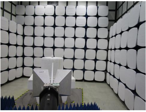
1.2 Radiated Spurious Emissions Test Setup
