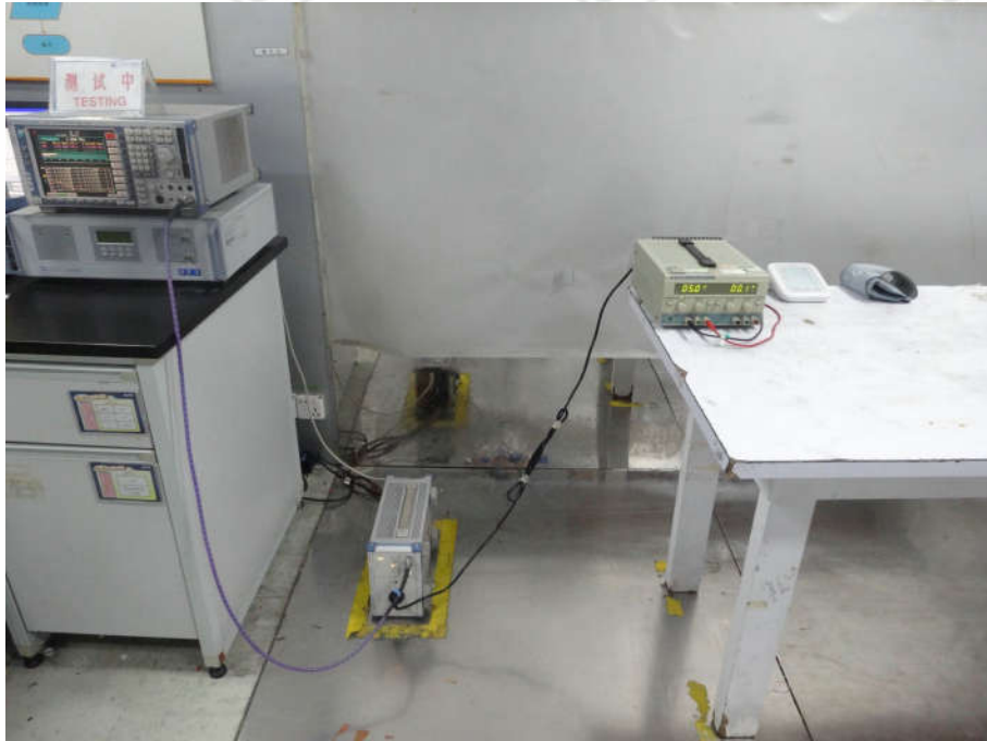
Conducted Emissions Test Setup
