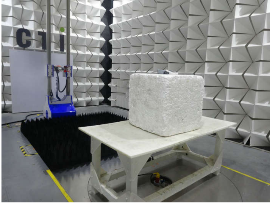
Radiated spurious emission Test Setup-3( Above 1G)
