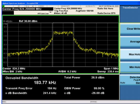
NB-IOT Band 5 QPSK 15kHz 12@0 CH-Middle
