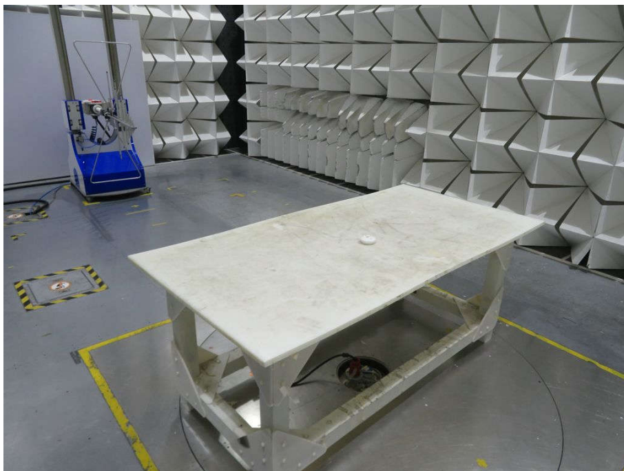
Radiated spurious emission Test Setup-2(Below 1GHz)
