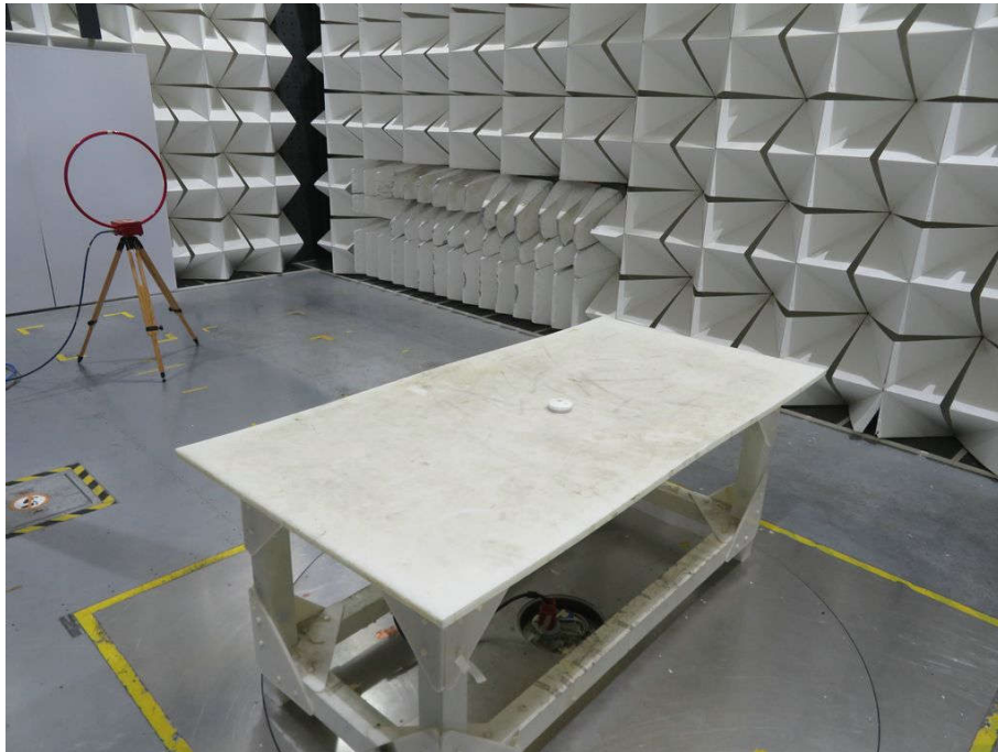
Radiated spurious emission Test Setup-1(Below 30MHz)
