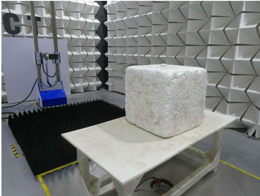
Radiated spurious emission Test Setup-3(Above 1GHz)
