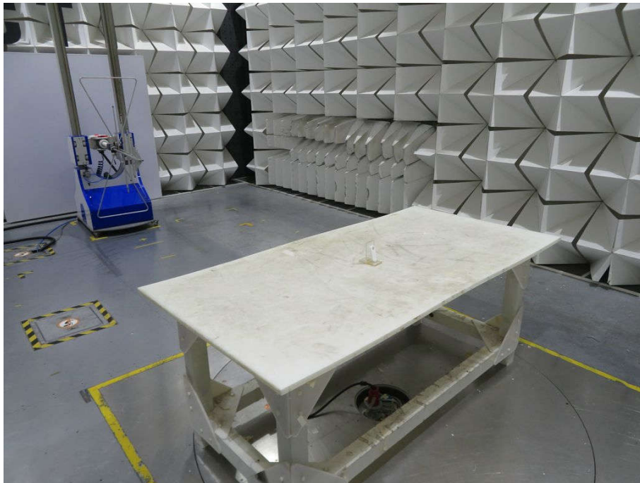
Radiated spurious emission Test Setup-2(Below 1GHz)
