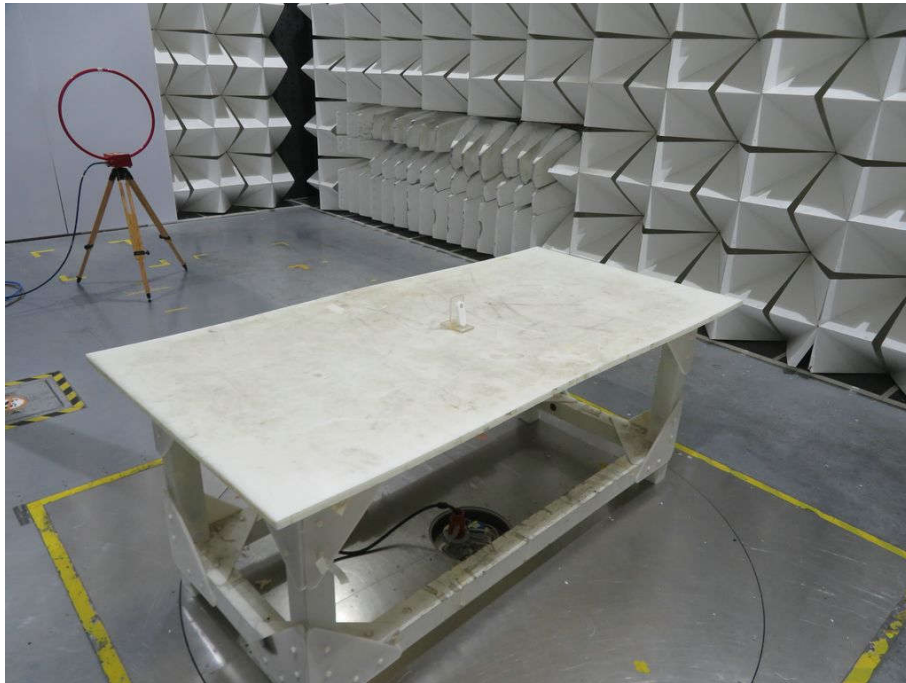
Radiated spurious emission Test Setup-1(Below 30MHz)
