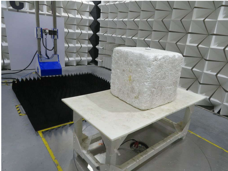
Radiated spurious emission Test Setup-3(Above 1GHz)
