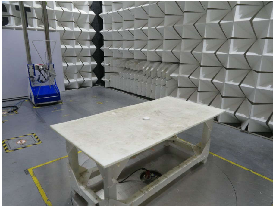
Radiated spurious emission Test Setup-2(Below 1GHz)
