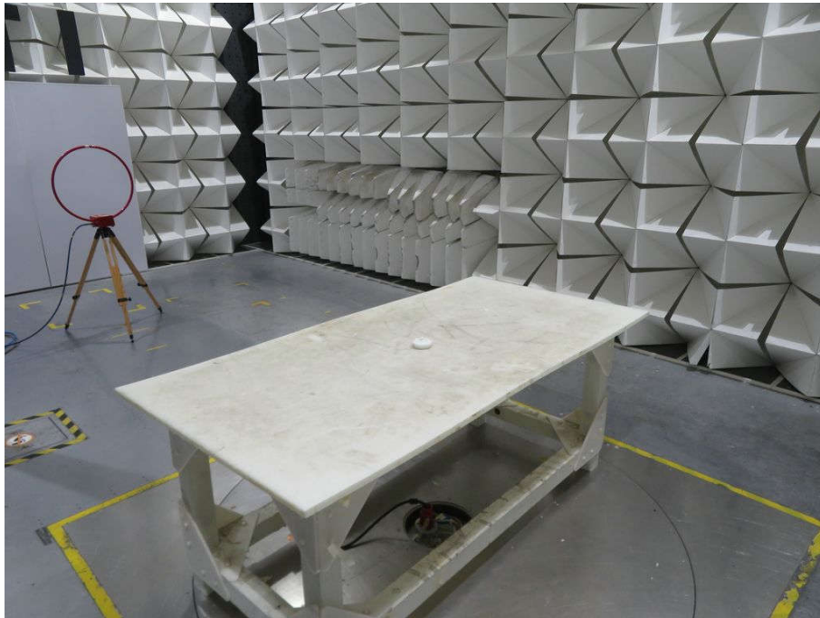
Radiated spurious emission Test Setup-1(Below 30MHz)
