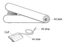
Connection: Insert the air plug of cuff air tube into air jack of the Electronic Blood Pressure Monitor. Figure as shown above.
