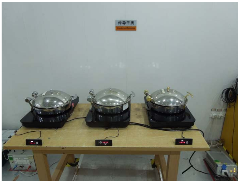
Photo of Setup for Conducted Emission (Three Unit)
