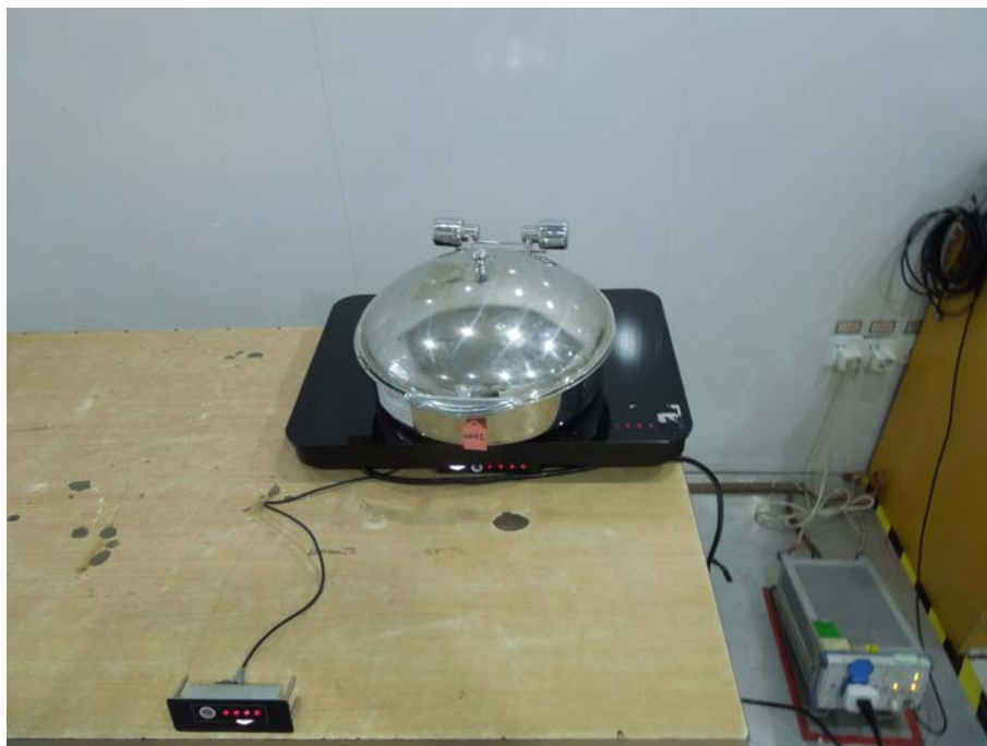
Photo of Setup for Conducted Emission (Three Unit)
