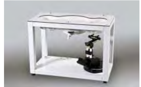
Figure E.5.1 SAM Twin Phantom
