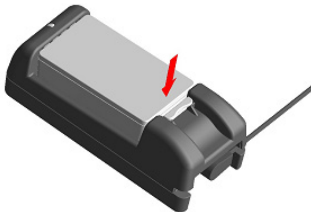
Figure 17-6 Battery Pack Installation (2)
