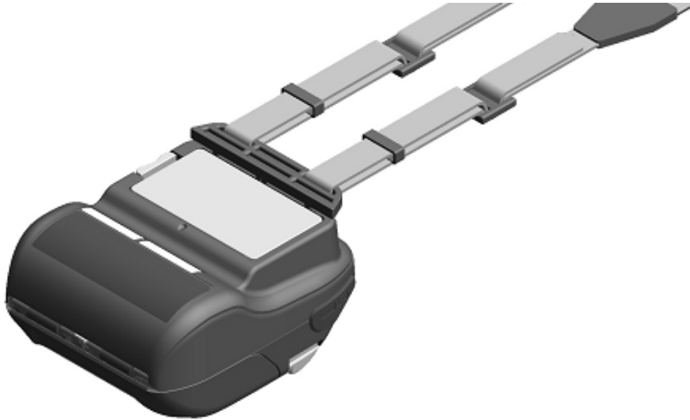
Figure 13-9 Shoulder Strap Installation (5)
