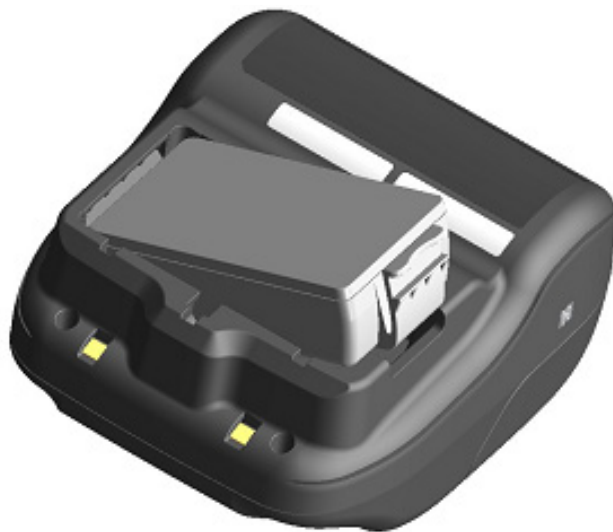
Figure 8-2 Installing Battery Pack (1)
