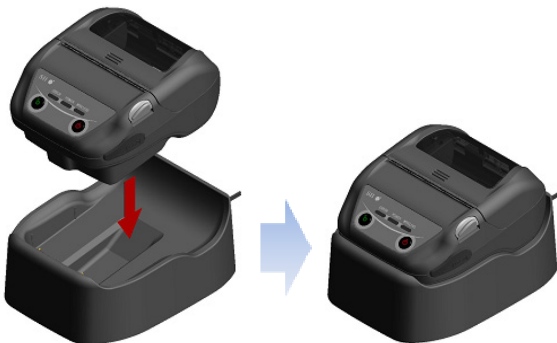
Figure 15-3 Printer and Cradle Connection
