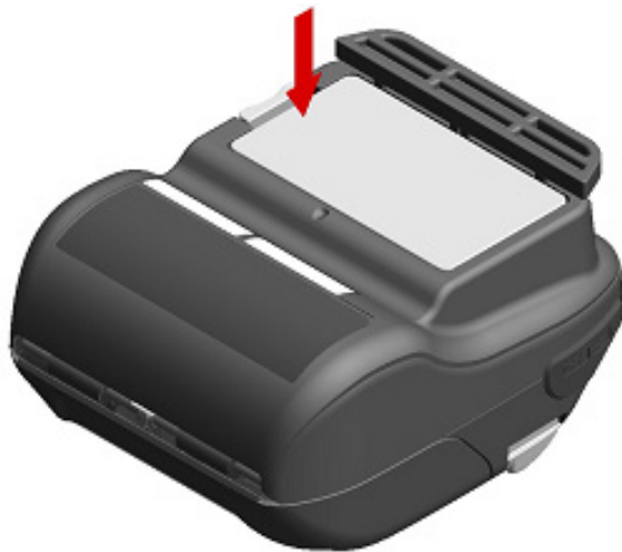
Figure 13-6 Shoulder Strap Installation (2)
