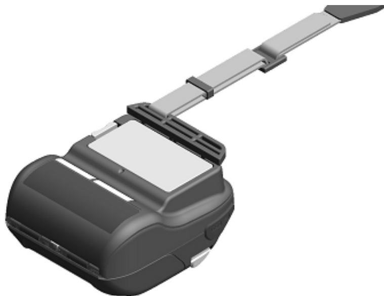
Figure 13-8 Shoulder Strap Installation (4)
