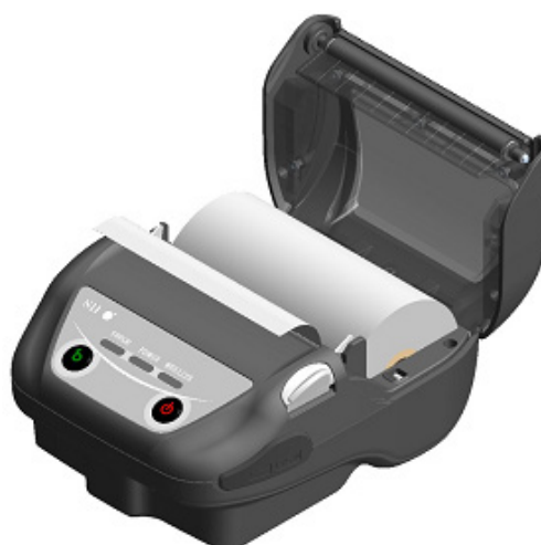
Figure 9-3 Thermal Paper Setting State
