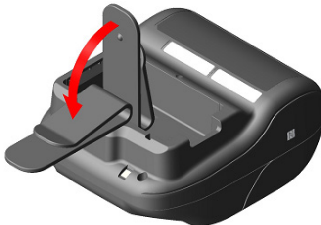
Figure 13-2 Belt Clip Installation (2)
