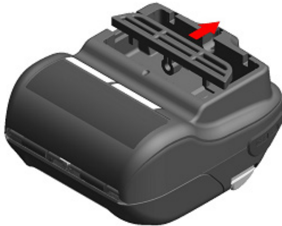
Figure 13-5 Shoulder Strap Installation (1)
