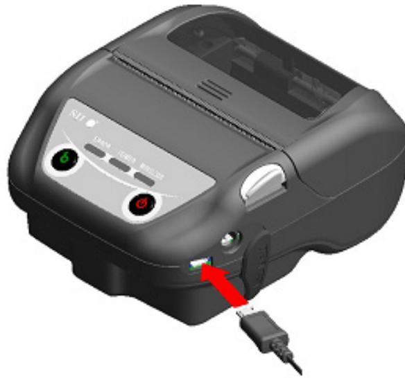
Figure 12-1 Printer and USB Cable Connection
