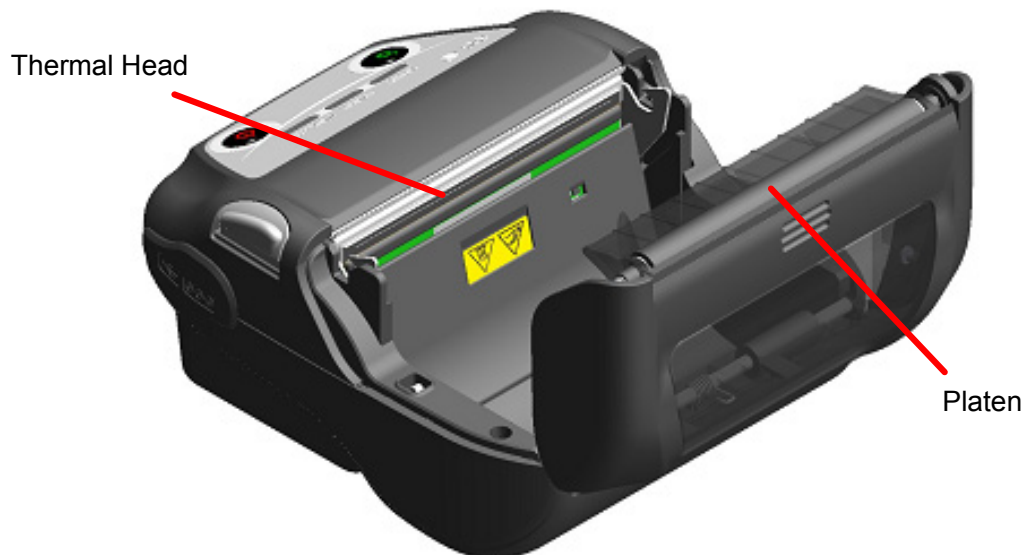
Figure 18-1 Cleaning Thermal Head / Platen
