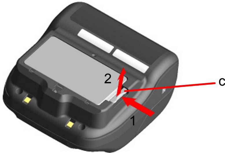
Figure 8-4 Removing Battery Pack
