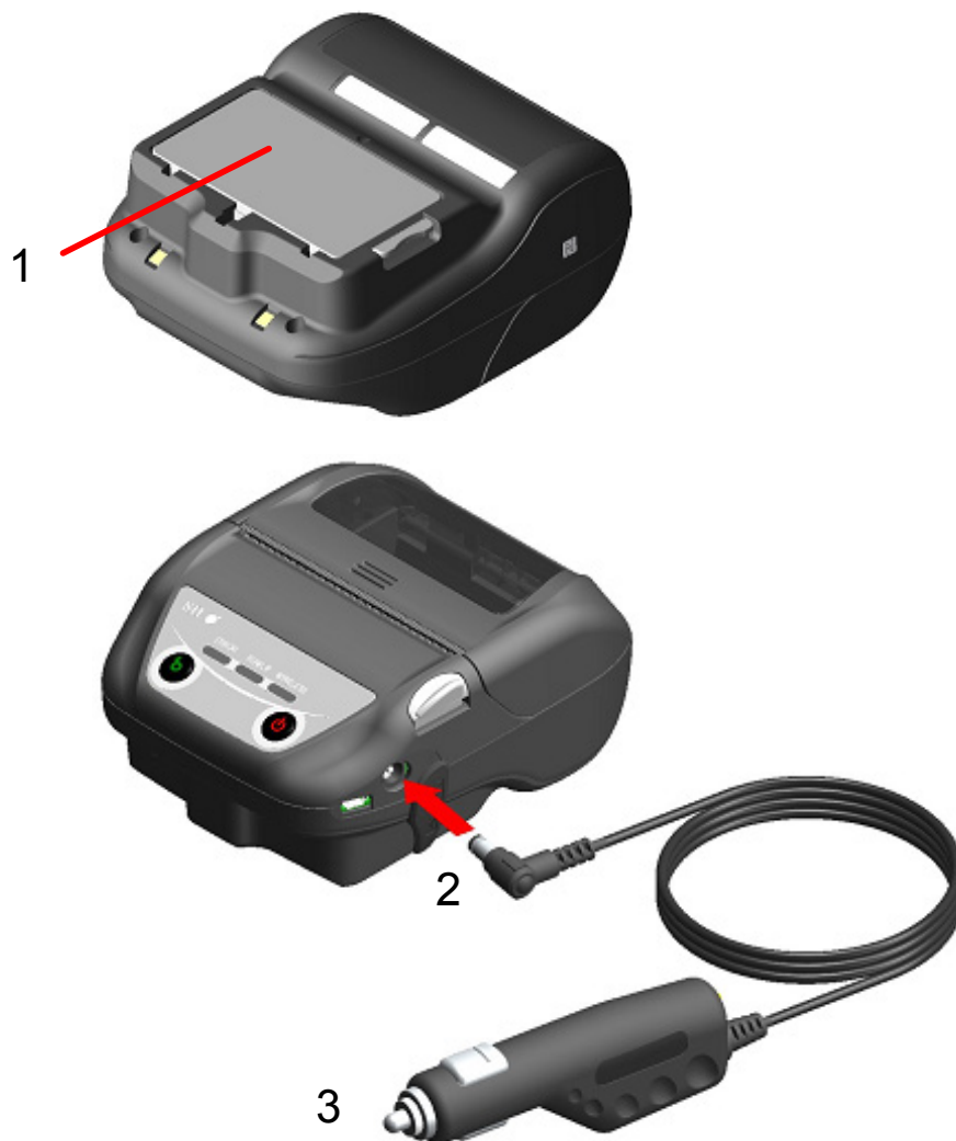
Figure 16-3 Charging in Power Off Charging Mode by Car Charger
