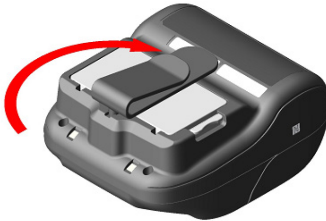
Figure 13-4 Belt Clip Installation (4)
