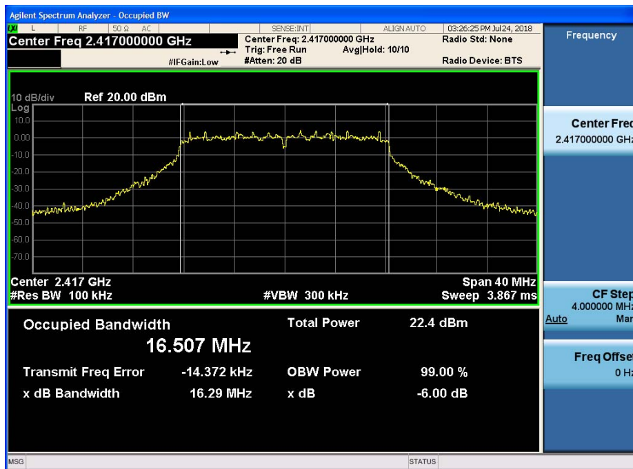
6dB Bandwidth plot (802.11g-CH 2)
