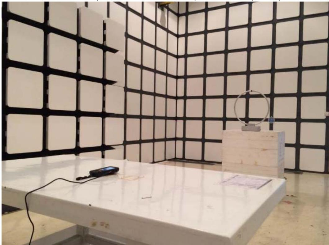
Radiated Spurious Measurement(30MHz to 1GHz) Setup
