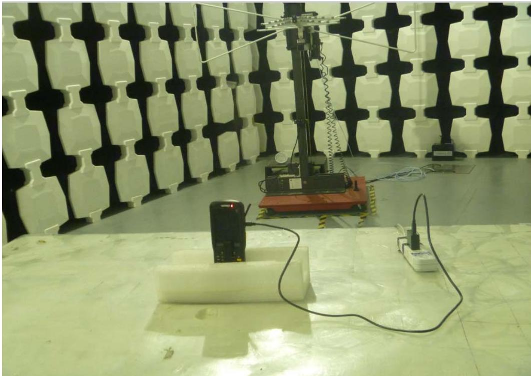
Radiated Spurious Measurement (Above 1GHz) Setup
