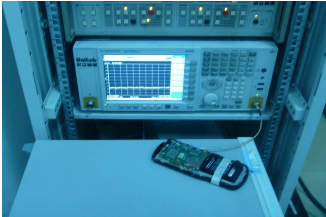
Radiated Spurious Measurement(Blow 30MHz) Setup
