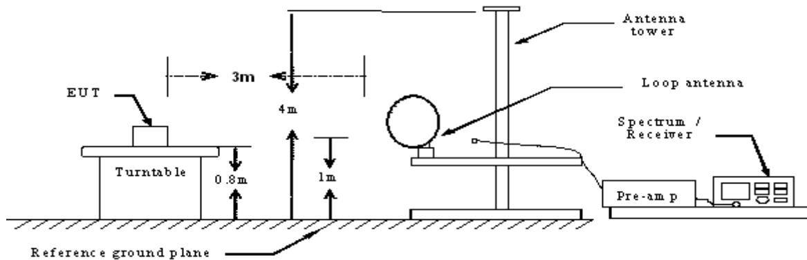
Radiated Spurious Measurement: below 1GHz
