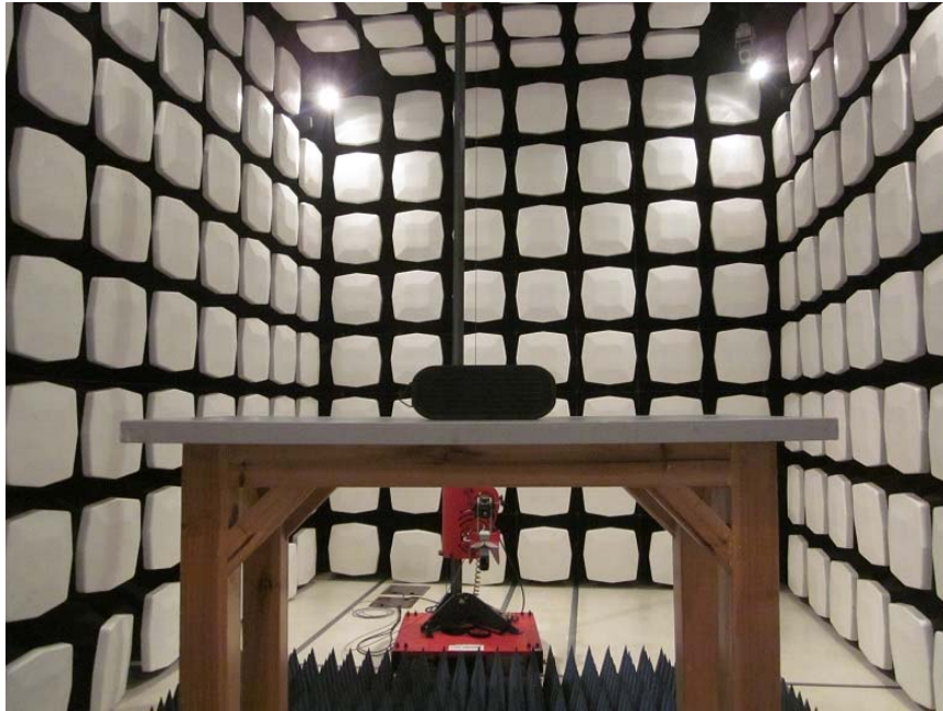
Measurement of Radiated Emission Test Set Up
