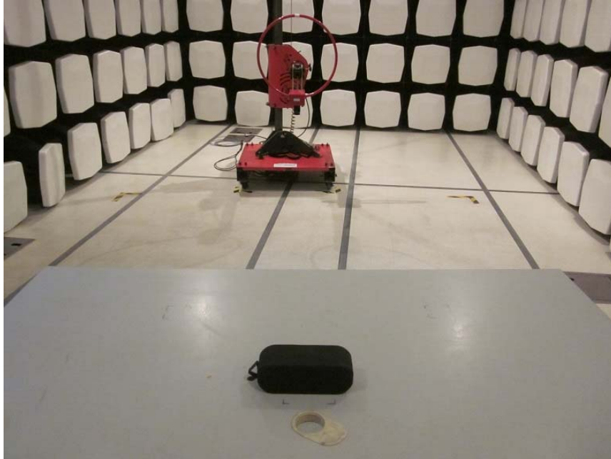
Measurement of Radiated Emission Test Set Up
