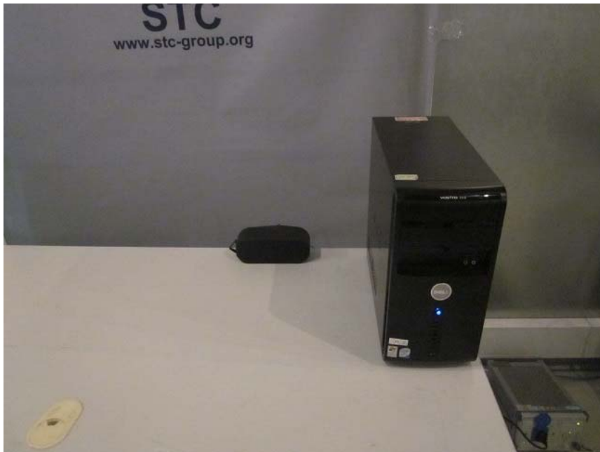
Measurement of Conducted Emission Test Set Up
