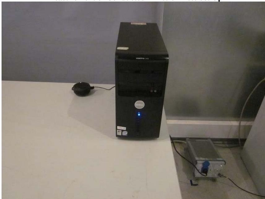
Measurement of Conducted Emission Test Set Up
