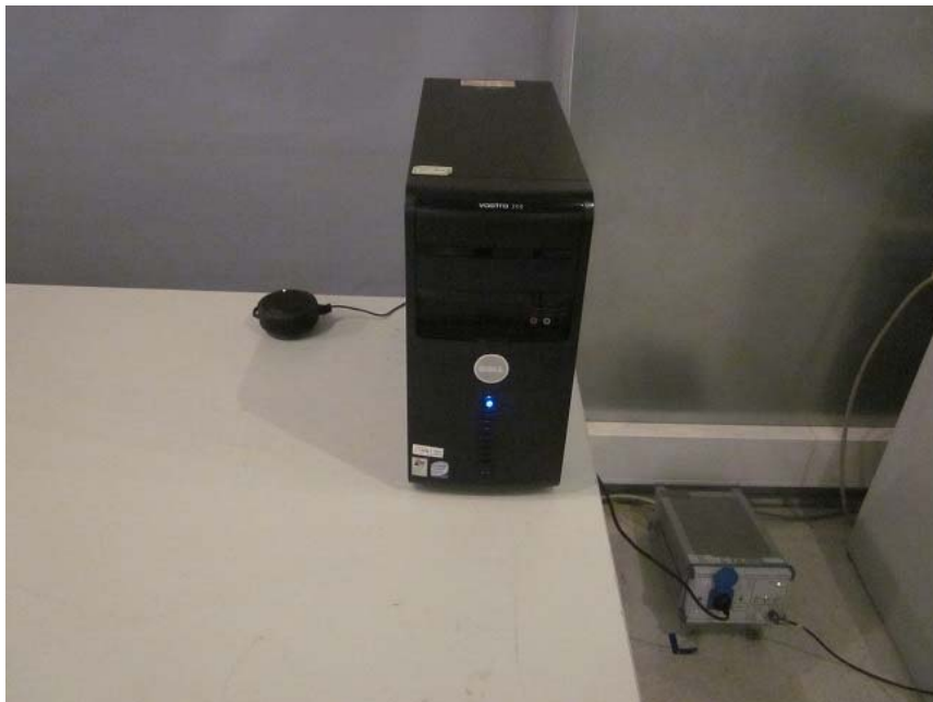
Measurement of Conducted Emission Test Set Up
