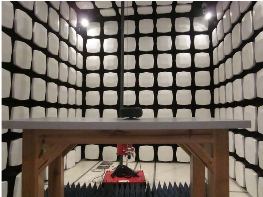
Measurement of Radiated Emission Test Set Up
