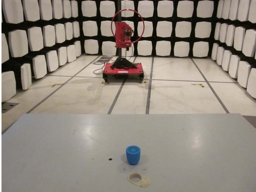
Measurement of Radiated Emission Test Set Up
