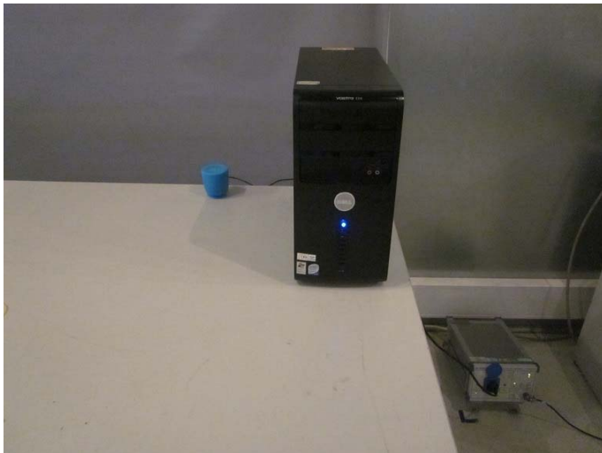
Measurement of Conducted Emission Test Set Up
