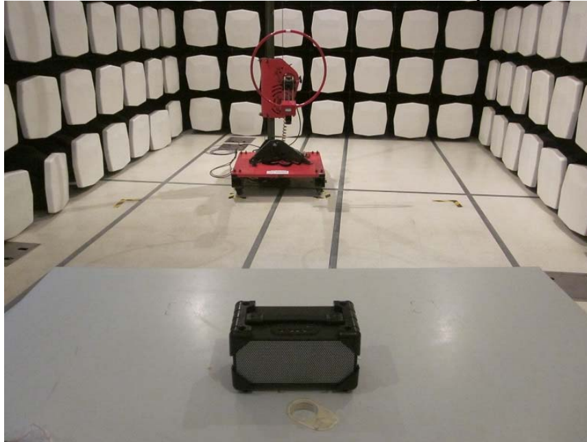
Measurement of Radiated Emission Test Set Up
