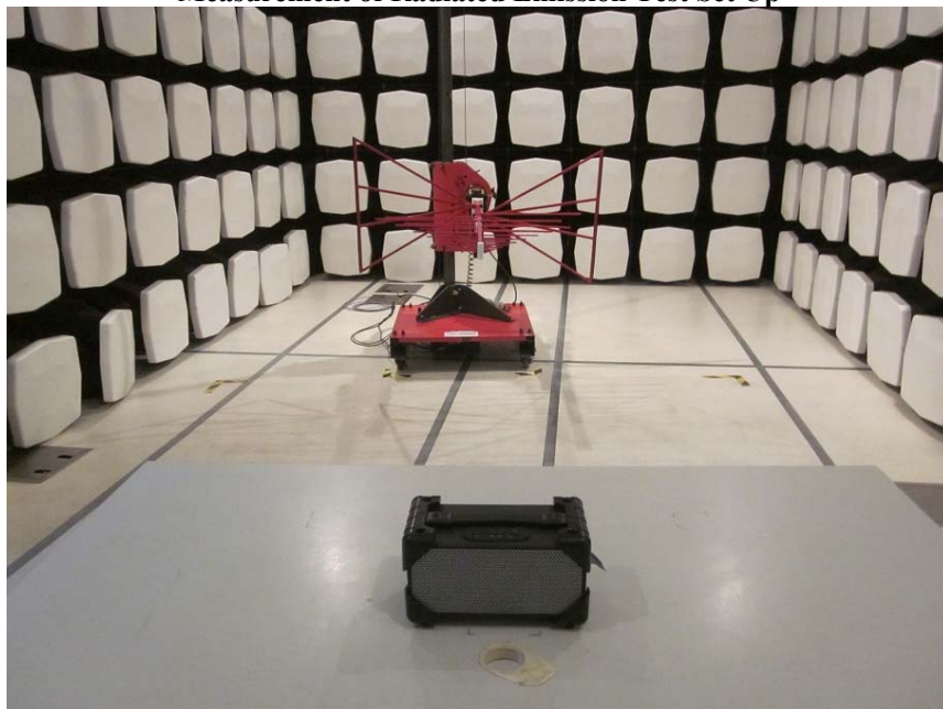
Measurement of Radiated Emission Test Set Up
