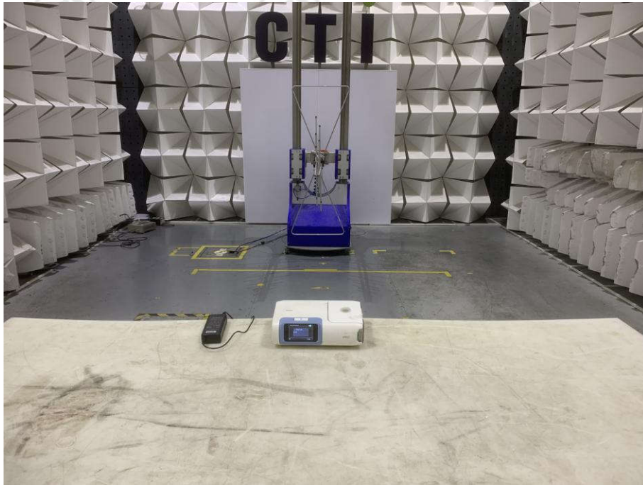
Radiated spurious emission Test Setup-1(Below 1GHz)
