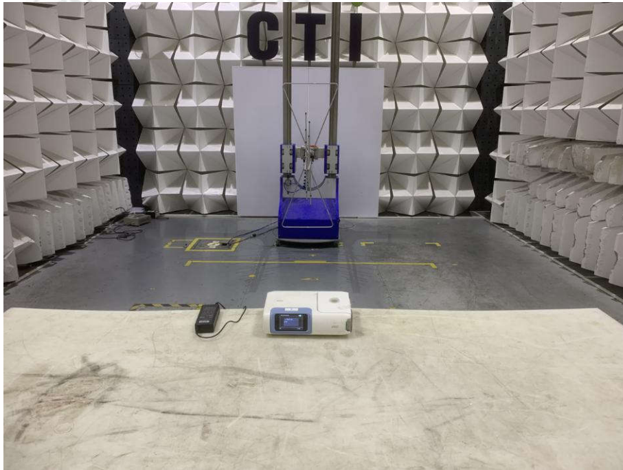
Radiated spurious emission Test Setup-1(Below 1GHz)
