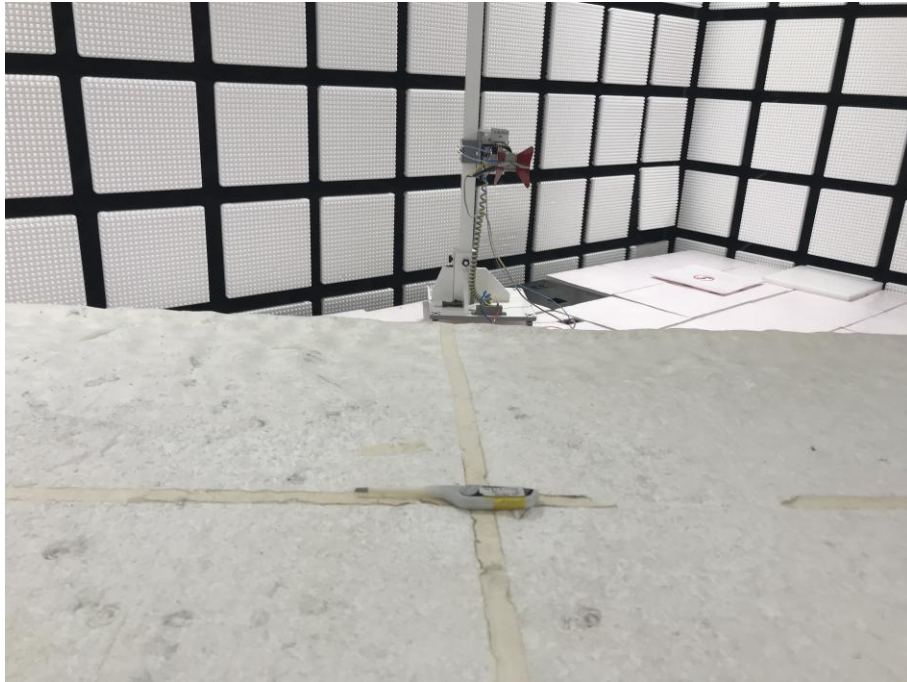
Radiated spurious emission Test Setup-2(Above 1GHz)Close up photos
