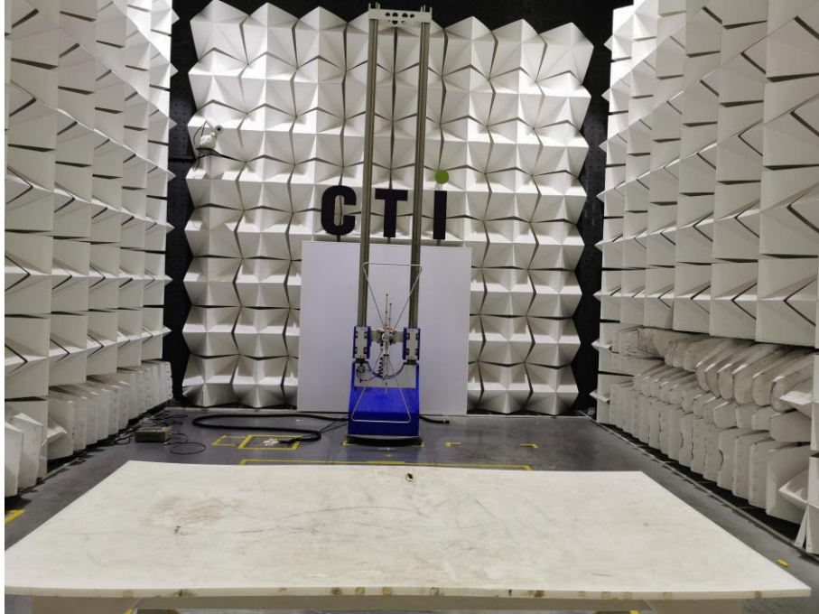
Radiated spurious emission Test Setup-1(Below 1GHz)
