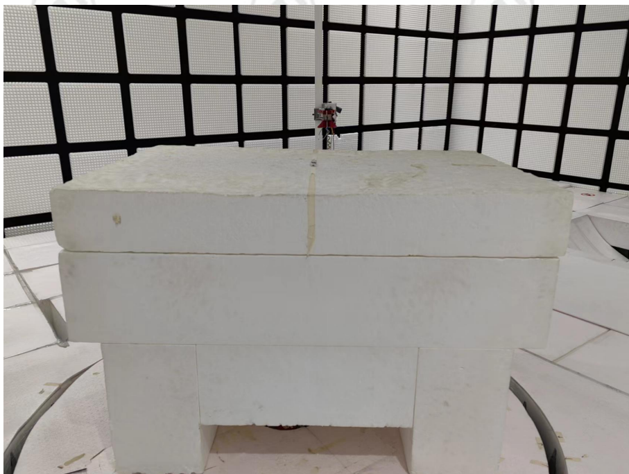
Radiated spurious emission Test Setup-2(Above 1GHz)
