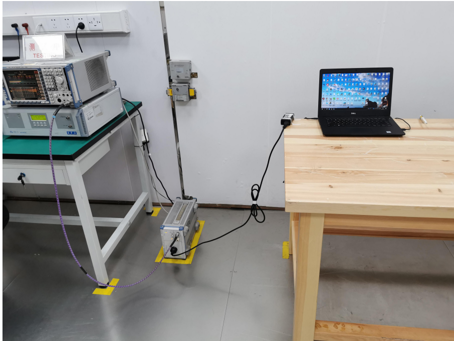
Conducted Emission Test Setup
