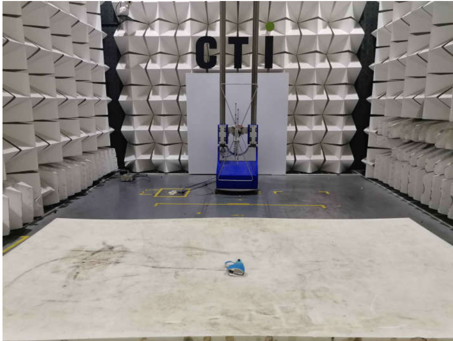
Radiated spurious emission Test Setup-1(Below 1GHz)
