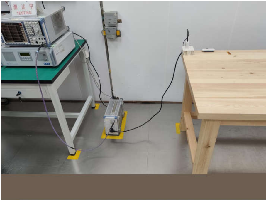
Conducted Emissions Test Setup
