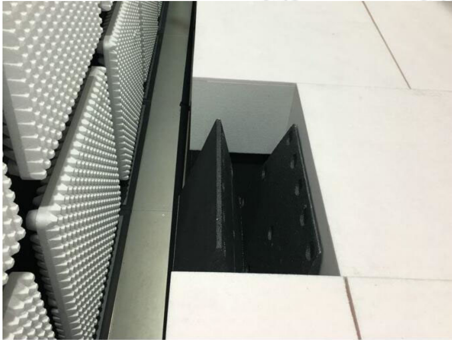
Radiated spurious emission Test Setup-5(Above 1GHz) There are absorbing materials under the ground.
