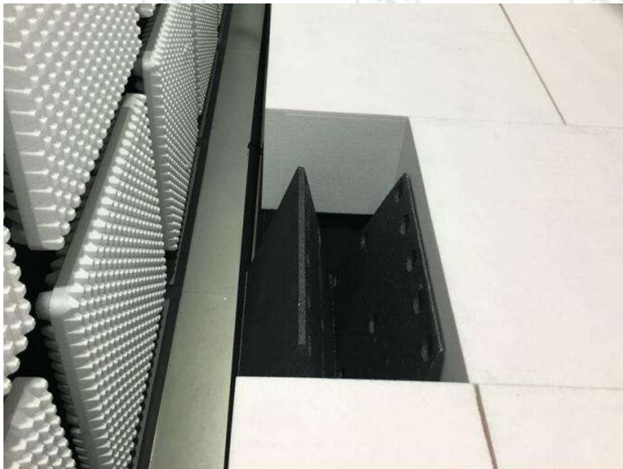
Radiated spurious emission Test Setup There are absorbing materials under the ground.
