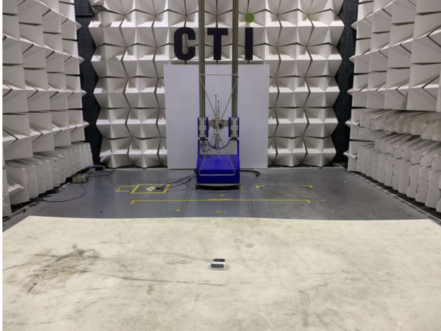
Radiated spurious emission Test Setup-1(Below 1GHz)
