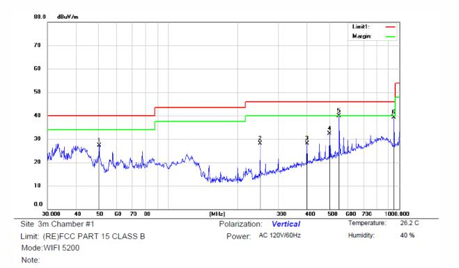
Reading Correct Measure-Antenna Table Freq. Limit Over No. Mk Level Factor ment Height Degree MHz dBuV dB dBuV/m dBuV/m dB Detector cm degree Comment 1 50.3647 39.34 -11.96 27.38 40.00 -12.62 QP -11.23 2 250.0820 39.30 28.07 46.00 -17.93 QP 3 400.0810 34.40 -6.35 28.05 46.00 -17.95 QP 37.26 4 500.0818 -4.93 32.33 46.00 -13.67 QP 5 549.9830 43.99 -4.03 39.96 46.00 -6.04 QP 6 950.4260 39.19 0.10 39.29 46.00 -6.71 QP
