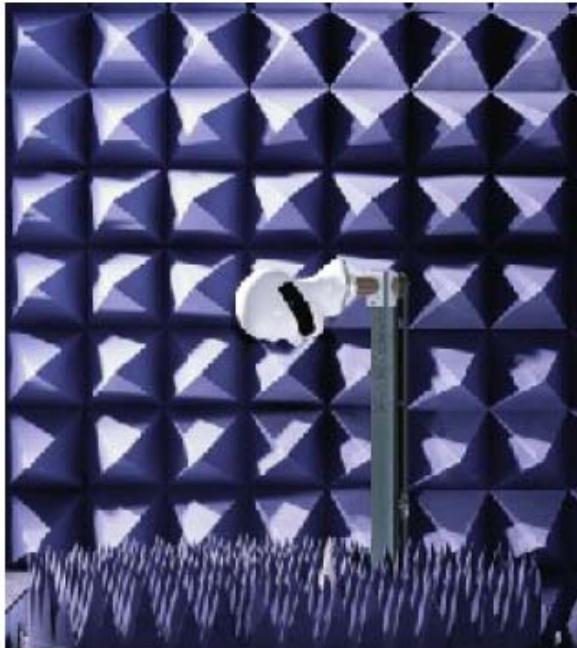
Figure 3: Typical test system showing 2115 medium duty MAPS on left and measurement antenna 3164-04 with the antenna set-up panel on right.
