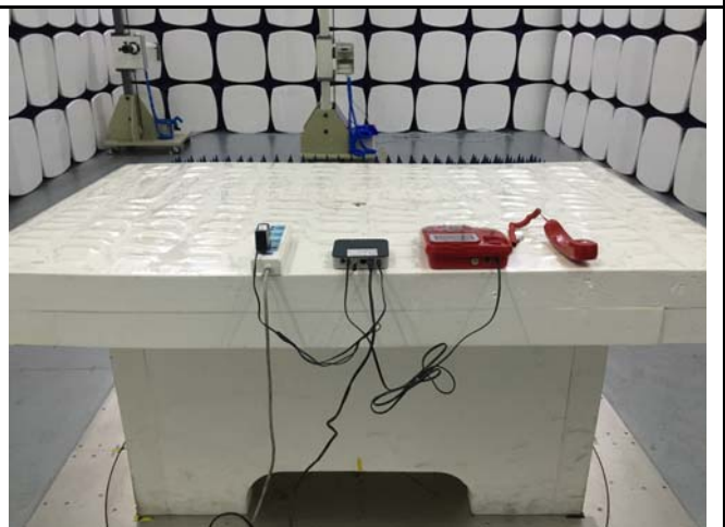
Radiated Emissions Test Setup Above 1GHz
