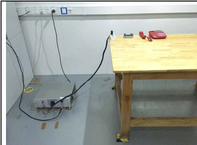
Conducted Emissions Test Setup – Front View
