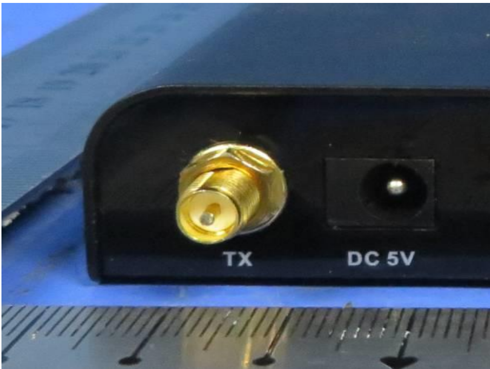
Close view for antenna port
