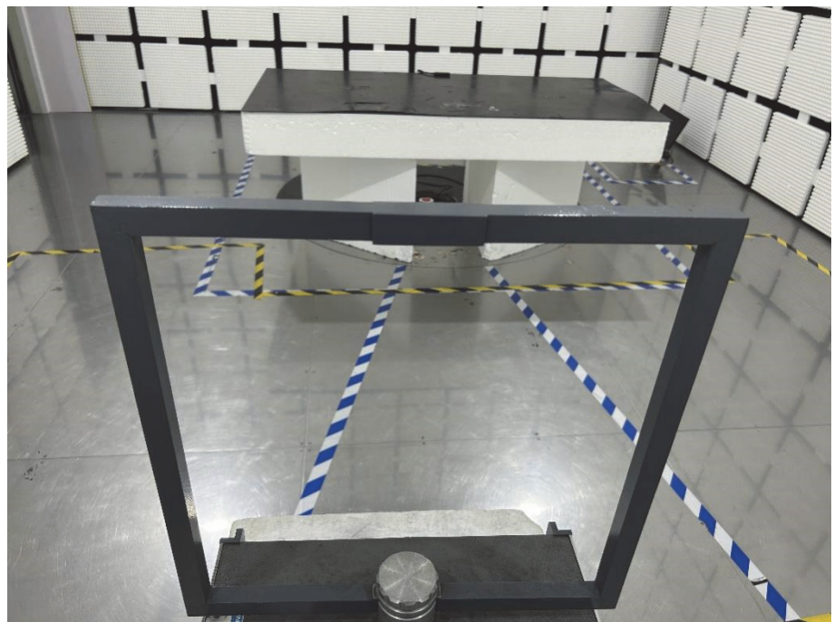
Radiation Emission Test Setup (Below 30MHz)
