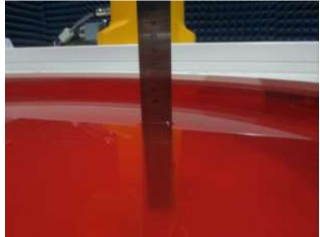
Fig. 9.6 Photo of Liquid Height for Body SAR of Twin Phantom (2450MHz) (depth>15cm)
