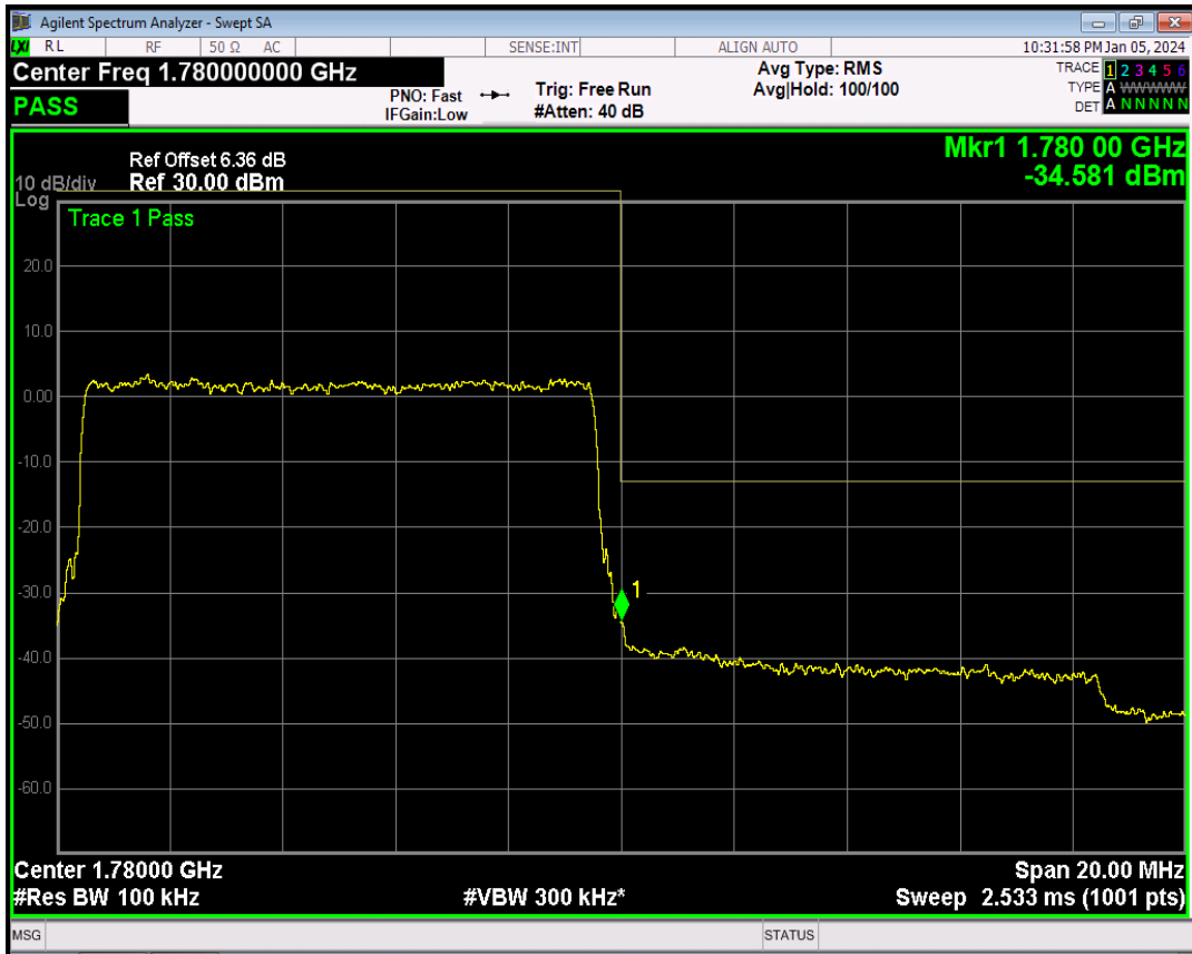
Band66 QPSK BW=10MHz Channel=132622 RB Size=50 Position=#0
