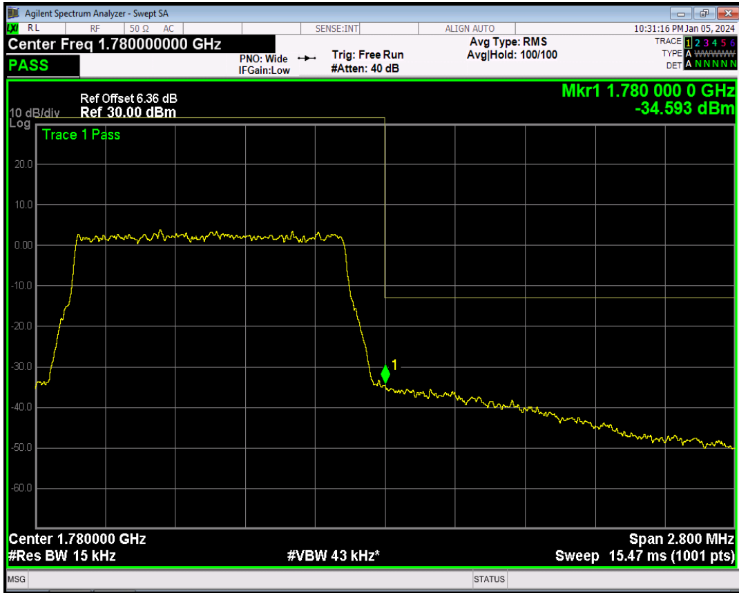
Band66 QPSK BW=3MHz Channel=131987 RB Size=15 Position=#0
