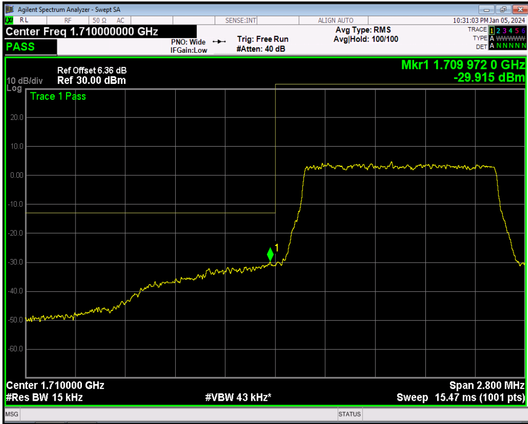
Band66 16QAM BW=1.4MHz Channel=131979 RB Size=6 Position=#0
