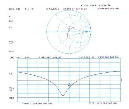
Impedance Measurement Plot for Body TSL
