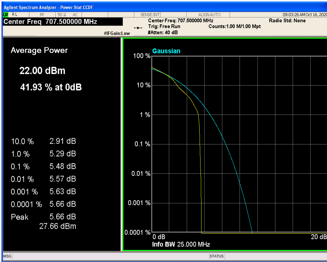
LTE Band12 QPSK BW=5MHz Channel=23095 RB Size=1 Position=#0
