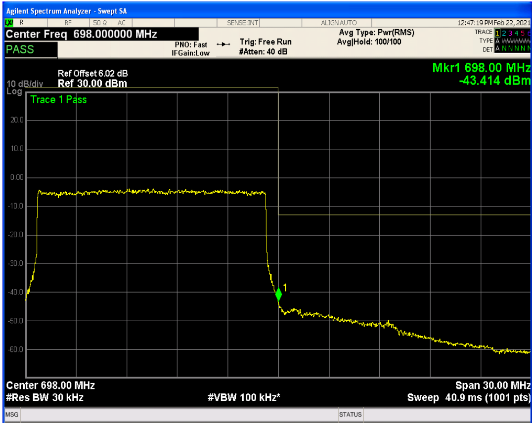
Band71 QPSK BW=20MHz Channel=133222 RB Size=1 Position=#Max
